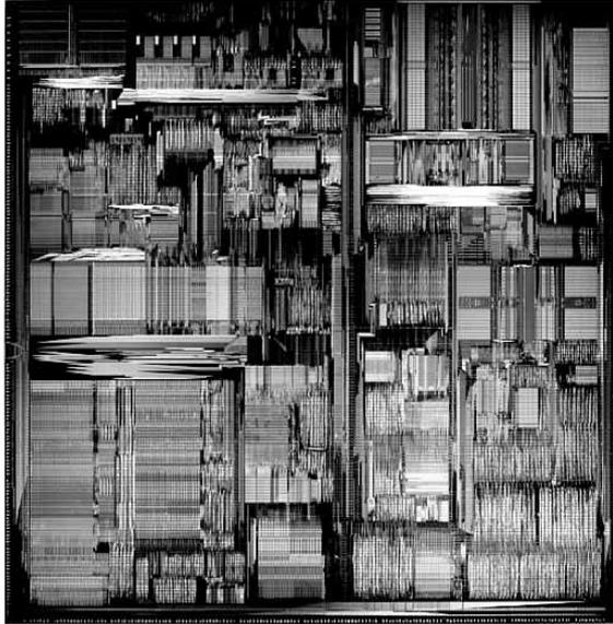
FIG. 3.22 Pentium Pro Processor die. *Photograph used by permission of Intel Corporation.*
