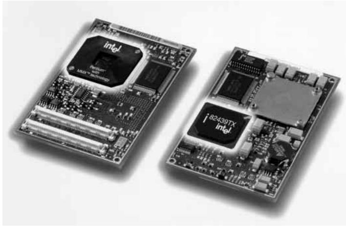
FIG. 15.10 Intel Pentium MMX mobile module, including the processor, chipset, and L2 cache. Photograph used by permission of Intel Corporation.
