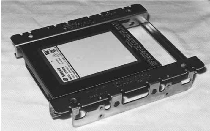
FIG. 12.13 A typical bracket used to mount a 3 1/2-inch drive in a 5 1/4-inch drive bay. The bracket is screwed to the drive and then mounted in the bay by using screws or rails as determined by the case.
