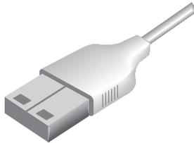
FIG. 10.5 The slots on the USB plug snap it into place on the spring-loaded tabs in a USB connector.
