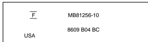
FIG. 5.8 The markings on a typical older memory chip.
