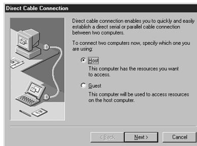
FIG. 11.3 Windows 9x enables you to access another computer using a serial or parallel connection.
