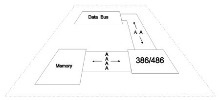
In view of the above, you can see that processor speed alone is no guide to performance, and in some cases may even be irrelevant. A slow hard disk (on the data bus), for instance, will always make any processor wait for its data and waste cycles that could be used for serious work. In fact, as far as NetWare is concerned, a 486/33 is only noticeably better than a 386 when network loading is heavy.
