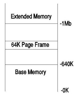
can be allocated to a program, but only one will be in the address space of the CPU at any time, as that bank is switched, or *paged*, in as required. In other words, the program code stays in the physical cells, but their electronic address is changed, either by software or circuitry.
