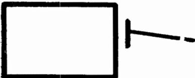
A barred tail always denotes control exit, which automatically maintains the entry interface of this module for reentry at next-sequential-statement.
