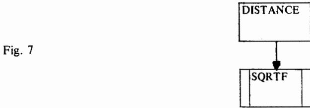
The data being passed as arguments are shown as an annotation to the connection for a "call." The small annotating arrow shows the direction of *flow* of the data. Thus
