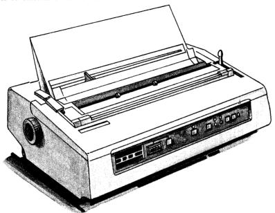
The letter-quality printer offers a choice of printing fonts and the option of a bidirectional forms tractor or a single or dual sheet feeder. The forms tractor feeds continuous fan fold paper. Both sheet feeders store and feed single-cut sheet paper, eliminating the need for fan fold paper or forms and making it possible to print on your own letterhead stationery.
