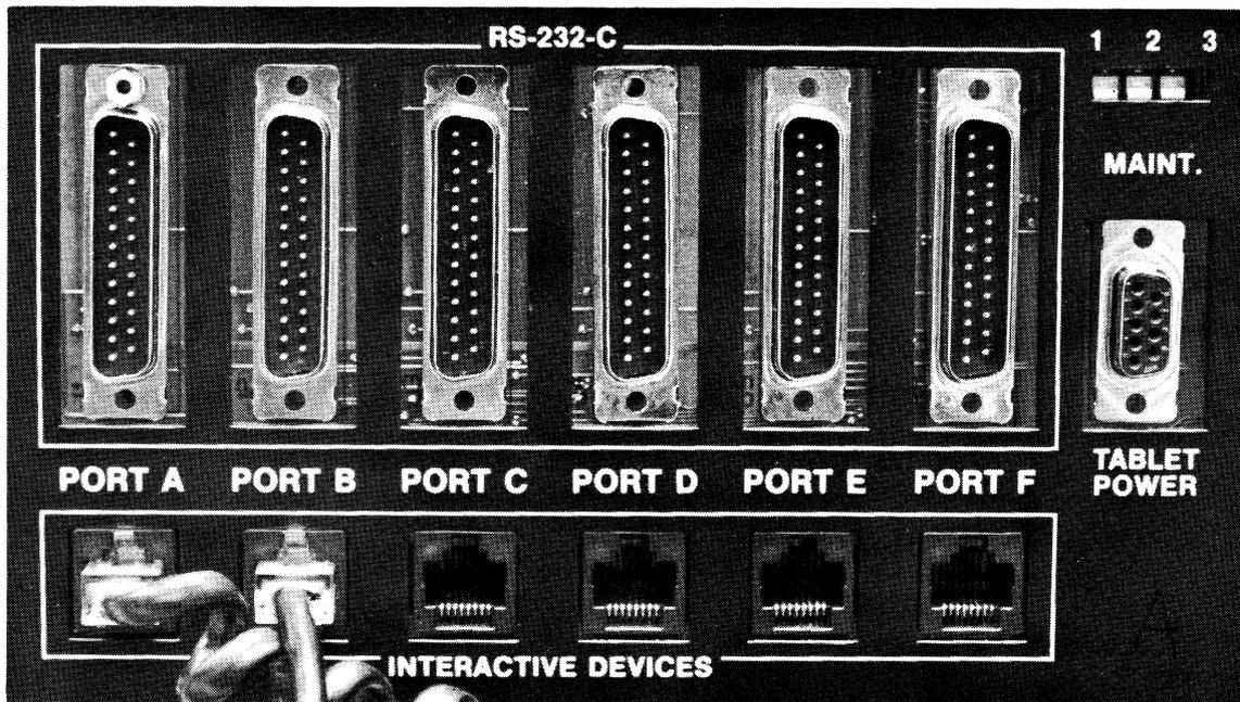
Figure 2-1. Port A of the Data Concentrator
