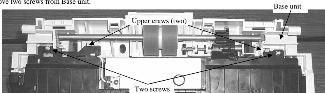
(4) Release two upper craws and two lower craws, and then remove Dust cover taking care that the cables from Dust cover shall not be pulled by force.
