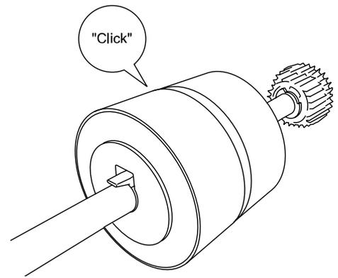
7. Attach the Pick roller shaft to the scanner.
