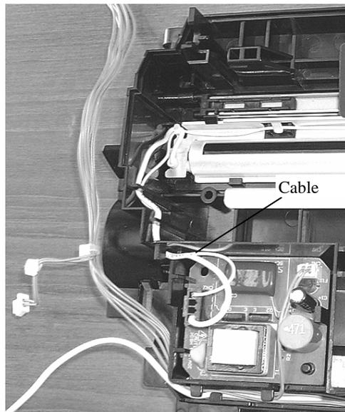
Note 2: When connecting a cable to Cover open sensor, a cable band shall be placed on U-shape slot of the frame. This cable setting is important to avoid the cable be disconnected by pulling the cable at assembling the scanner later. Long-nose pliers may be necessary to connect the cable to Cover open sensor.
