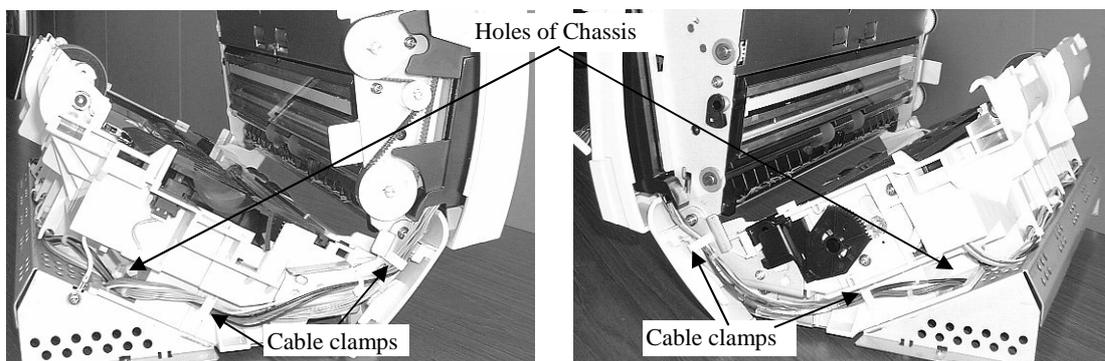
Note: Route the cables as shown in above figures when assembling.
