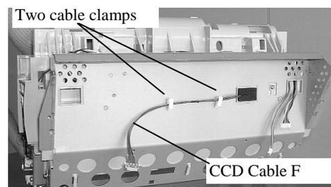
(4) Lift up the Optical unit while gently pulling CCD cable F through a slot of rubber. Finally push the connector of CCD cable F by your finger to remove Optical unit (OPT Unit with Cable F).
