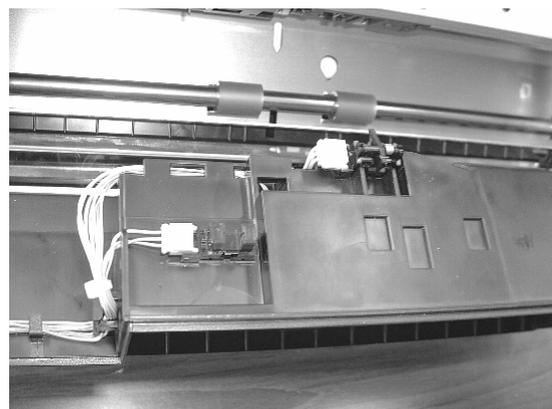
(6) Release the craws that fix the sensors and disconnect the connector of the sensor to remove.
