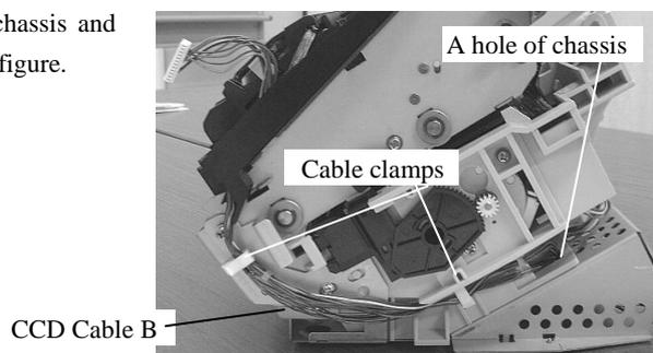
(3) Also remove CCD Cable B from the hooks of upper unit, shown in the bottom right figure, and then remove "OPT unit with Cable B" upward.
