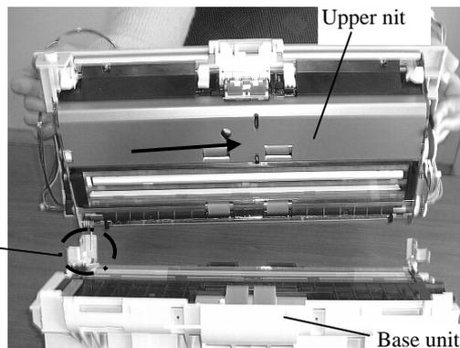
Note: When assembling the Upper unit, insert an arm of coil spring into a slot of bracket first, and insert the shaft to the hole of bracket as shown in the figure below. Then attach a plastic washer to another end of the shaft, and then insert the shaft into a hole of bracket as shown in the right figure. If a plastic washer is not inserted, the backside image may shift horizontally.
