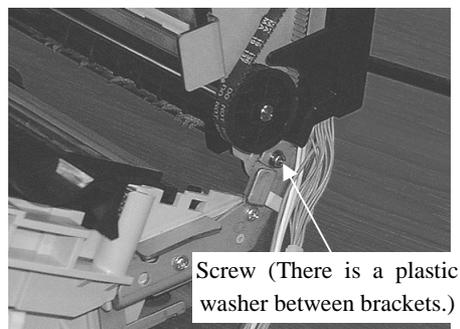
(4) Insert a small flat screwdriver between the brackets of fulcrum near the pulley, and then remove the shaft from the bracket of Base unit. Do not loose a plastic washer, which is located between the brackets.
