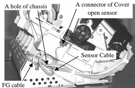
(3) Remove two screws from Base unit.
