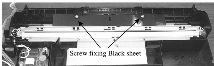
(4) Release three craws A that fix the Reflector of the lamp.
