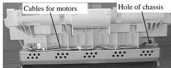
(4) Remove two screws from PICK Motor, and remove the motor.
