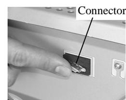
(5) Remove the CCD Cable F from the Optical unit by releasing the cable from the hooks and disconnecting the connector.
