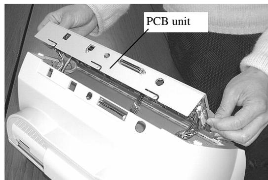
(3) Disconnect 8 connectors, which are connected to the PCB Unit, and remove the PCB Unit. To replace Control PCA, go to [Section 4-11](#).
