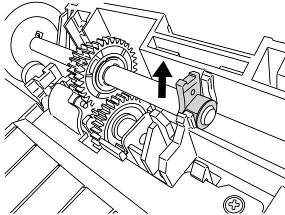
Note: As the Pick roller bushing is firmly fixed, do not try to turn the roller bushing with your fingernails. Use a paper clip for the roller bushing if you cannot rotate it with your finger.
