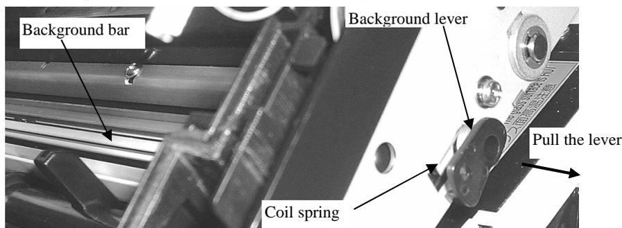
Note: Mounting procedure of the Background bar and Background lever is as follows.
