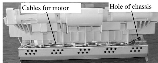
(4) Remove two screws that are fixing the BW motor. Slide the motor inside and tilt it to remove the motor from the Upper unit.
