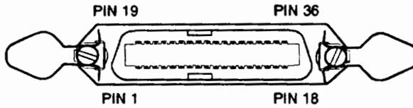
**Parallel Interface 36-pin Panel Mount Receptacle
