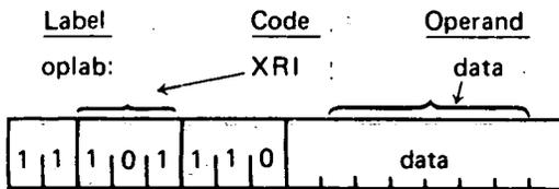
Description: The byte of immediate data is EXCLUSIVE-ORED with the contents of the accumulator. The carry bit is set to zero.
