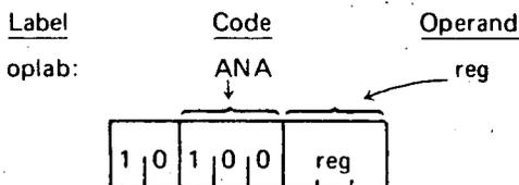
Description: The specified byte is logically ANDed bit by bit with the contents of the accumulator. The Carry bit is reset to zero.
