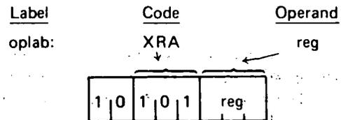
Description: The specified byte is EXCLUSIVE-ORed bit by bit with the contents of the accumulator. The Carry bit is reset to zero.
