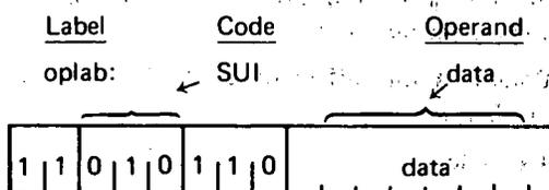
Description: The byte of immediate data is subtracted from the contents of the accumulator using two's complement arithmetic.
