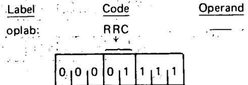
Description: The carry bit is set equal to the low-order bit of the accumulator. The contents of the accumulator are rotated one bit position to the right, with the low-order bit being transferred to the high-order bit position of the accumulator.
