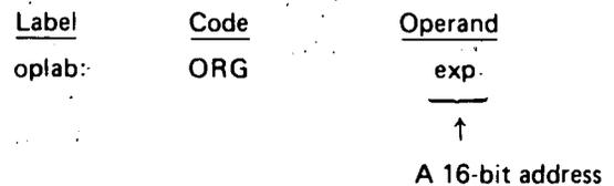
Description: The assembler's location counter is set to the value of exp, which must be a valid 16-bit memory address. The next machine instruction or data byte(s) generated will be assembled at address exp, exp+1, etc.
