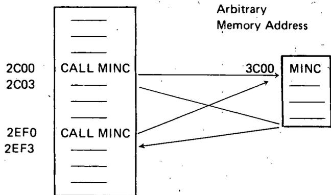
When the first call is executed, address 2C03H is pushed onto the stack indicated by the stack pointer, and control is transferred to 3C00H. Execution of either RETURN statement in MINC will cause the top entry to be popped off the stack into the program counter, causing execution to continue at 2C03H (since the CALL statement is three bytes long).
