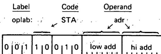
Description: The contents of the accumulator replace the byte at the memory address formed by concatenating HI ADD with LOW ADD.
