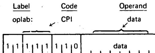
Description: The byte of immediate data is compared to the contents of the accumulator.
