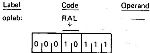
Description: The contents of the accumulator are rotated one bit position to the left.
