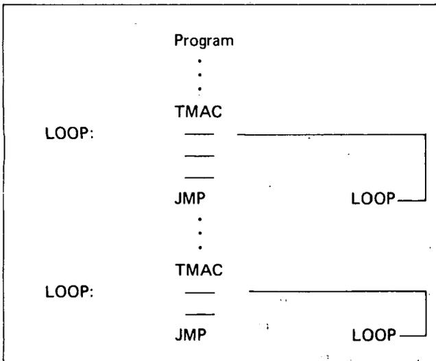
If in the macro definition, LOOP had been followed by two successive colons, LOOP would be generated as a global label by the first reference to TMAC, while the second reference would be flagged as an error.
