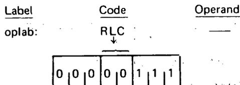
Description: The Carry bit is set equal to the high-order bit of the accumulator. The contents of the accumulator are rotated one bit position to the left, with the high-order bit being transferred to the low-order bit position of the accumulator.
