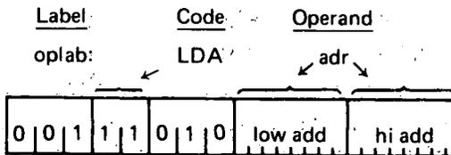
Description: The byte at the memory address formed by concatenating HI ADD with LOW ADD replaces the contents of the accumulator.
