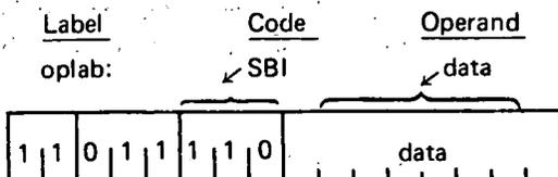
Description: The Carry bit is internally added to the byte of immediate data. This value is then subtracted from the accumulator using two's complement arithmetic.
