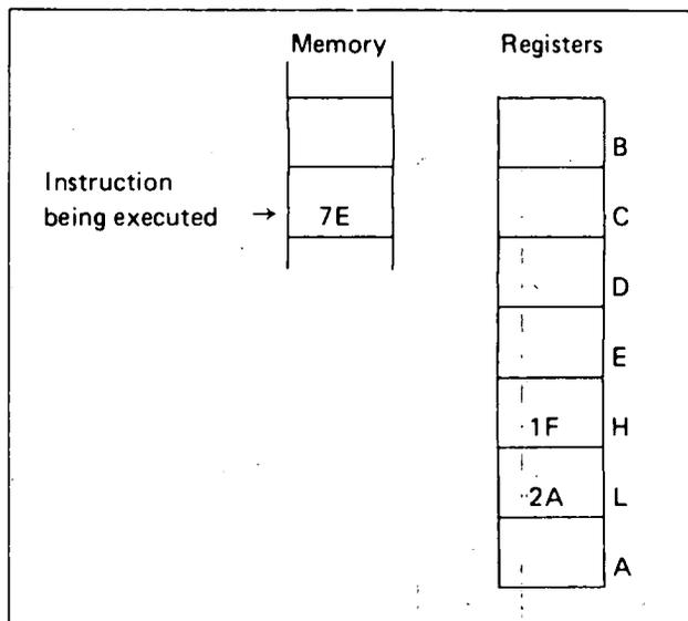
In addition, there are two 8080 instructions which use either the B and C registers or the D and E registers to address memory. As above, the first register of the pair holds the most significant 8 bits of the address, while the second register holds the least significant 8 bits. These instructions, STAX and LDAX, are described in Chapter 2 under Data Transfer Instructions.
