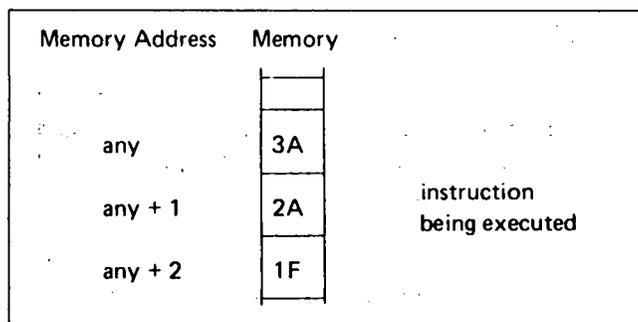
The instruction occupies three memory bytes, the second and third of which hold the direct address.
