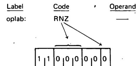
Description: If the Zero bit is zero, a return operation is performed.
