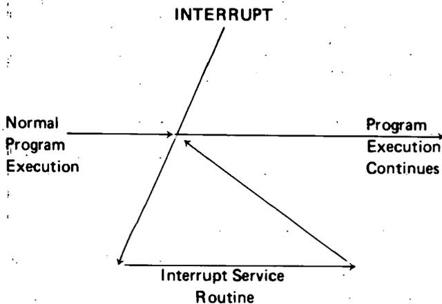
The 8080 contains a bit named INTE which may be set or reset by the instructions EI and DI described in Chapter 2. Whenever INTE is equal to 0, the entire interrupt handling system is disabled, and no interrupts will be accepted.
