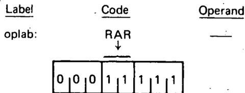
Description: The contents of the accumulator are rotated one bit position to the right.
