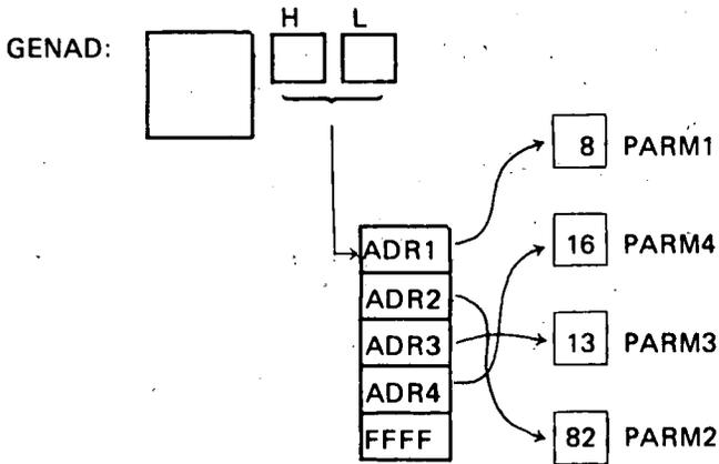
As implemented below, GENAD saves the current sum (beginning with zero) in the C register. It then loads the address of the first parameter into the D and E registers. If this address is greater than or equal to FF00H, it reloads the accumulator with the sum held in the C register and returns to the calling routine. Otherwise, it loads the parameter into the accumulator and adds the sum in the C register to the accumulator. The routine then loops back to pick up the remaining parameters.
