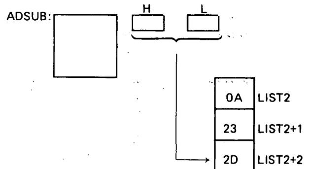
Note that the parameter lists PLIST and LIST2 could appear anywhere in memory without altering the results produced by ADSUB.
