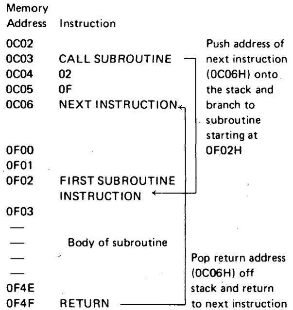
Subroutines may be nested up to any depth limited only by the amount of memory available for the stack. For example, the first subroutine could itself call some other subroutine and so on. An examination of the sequence of stack pushes and pops will show that the return path will always be identical to the call path, even if the same subroutine is called at more than one level.
