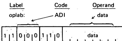
Description: The byte of immediate data is added to the contents of the accumulator using two's complement arithmetic.
