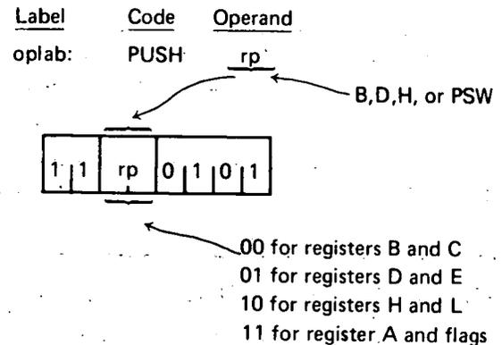
Description: The contents of the specified register pair are saved in two bytes of memory indicated by the stack pointer SP.
