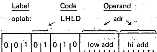
Description: The byte at the memory address formed by concatenating HI ADD with LOW ADD replaces the contents of the L register. The byte at the next higher memory address replaces the contents of the H register.
