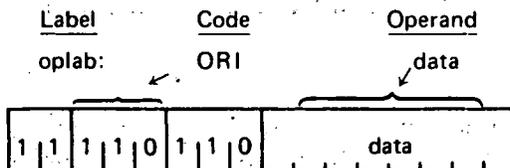
Description: The byte of immediate data is logically ORed with the contents of the accumulator.
