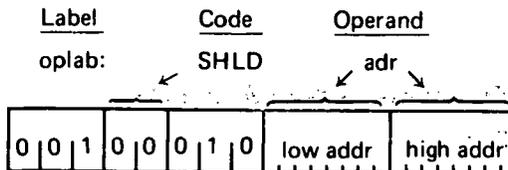
Description: The contents of the L register are stored at the memory address formed by concatenating HI ADD with LOW ADD. The contents of the H register are stored at the next higher memory address.
