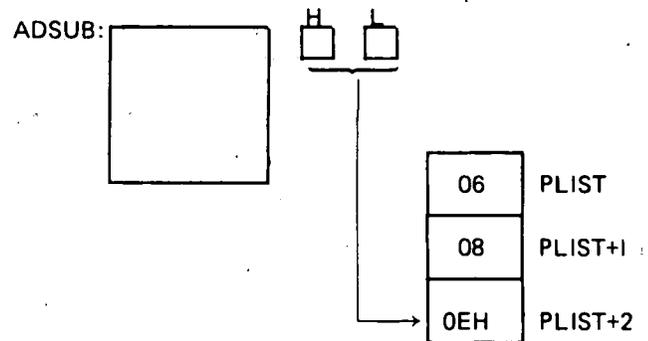
The second time ADSUB is called, the H and L registers point to the parameter list LIST2. The A and B registers are loaded with 10 and 35 respectively, and the sum is stored at LIST2 + 2. Return is then made to the instruction at RET2.
