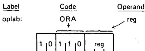
Description: The specified byte is logically ORed bit by bit with the contents of the accumulator. The carry bit is reset to zero.
