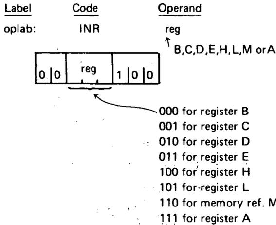
Description: The specified register or memory byte is incremented by one.
