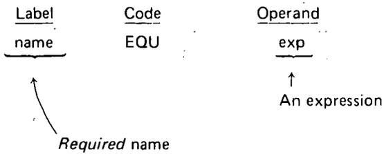
Description: The symbol "name" is assigned the value by EXP by the assembler. Whenever the symbol "name" is encountered subsequently in the assembly, this value will be used.
