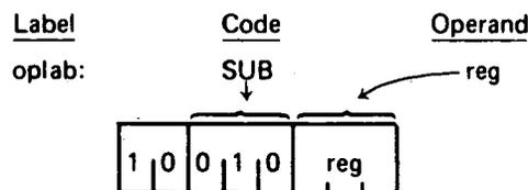
Description: The specified byte is subtracted from the accumulator using two's complement arithmetic.
