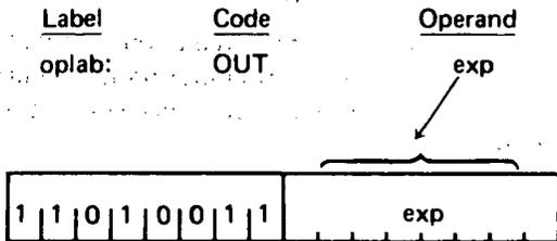
Description: The contents of the accumulator are sent to output device number exp.
