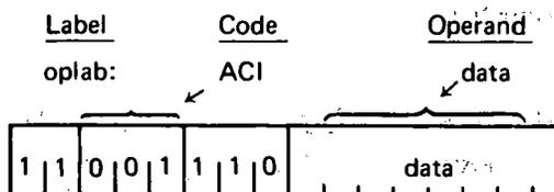
Description: The byte of immediate data is added to the contents of the accumulator plus the contents of the carry bit.
