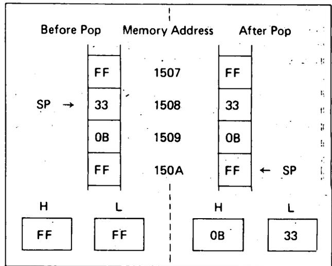
The programmer loads the stack pointer with any desired value by using the LXI instruction described in Chapter 2 under Load Register Pair-Immediate. The programmer must initialize the stack pointer before performing a stack operation, or erroneous results will occur.
