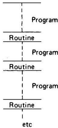
A more efficient means of accessing the routine would be to store it once, and find a way of accessing it when needed:
