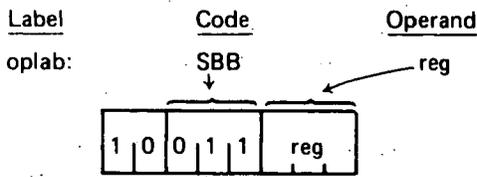
Description: The Carry bit is internally added to the contents of the specified byte. This value is then subtracted from the accumulator using two's complement arithmetic.
