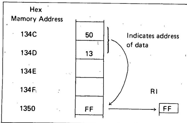
If the address of INADD is 134CH, register RI will be loaded from the address held in memory locations 134CH and 134DH, which is 1350H.
