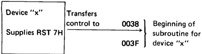
Note that any of these 8-byte subroutines may in turn call longer subroutines to process the interrupt, if necessary.
