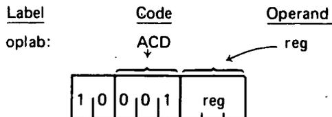
Description: The specified byte plus the content of the Carry bit is added to the contents of the accumulator.
