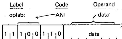
Description: The byte of immediate data is logically ANDed with the contents of the accumulator. The Carry bit is reset to zero.
