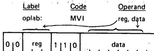
Description: The byte of immediate data is stored in the specified register or memory byte.
