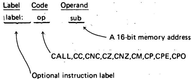
Instructions in this class call subroutines upon certain specified conditions. If the specified condition is true, a return address is pushed onto the stack and program execution
