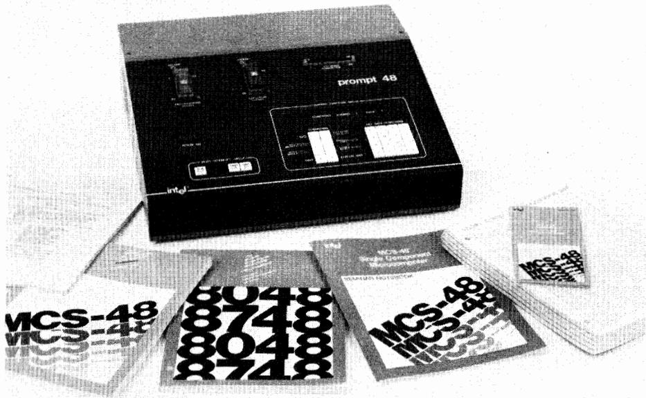
The 8748 is the first microcomputer fully integrated on one component. All elements of a computing system are provided, including CPU, RAM, I/O, timer, interrupts and erasable, reprogrammable non-volatile program memory.
