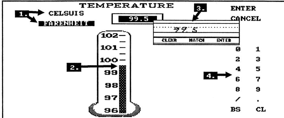
CODE-WRITE provides program access to the unique LINUS Pen-on-screen input/output routines. Four input methods are displayed: 1. Selection Buttons. 2. Point-and-enter. 3. Window for handwritten data. 4. Soft keypad.
