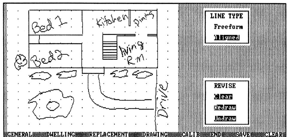
Computer aided drawings can now be generated and edited in the field. The pen can be used in places where a mouse can not.
