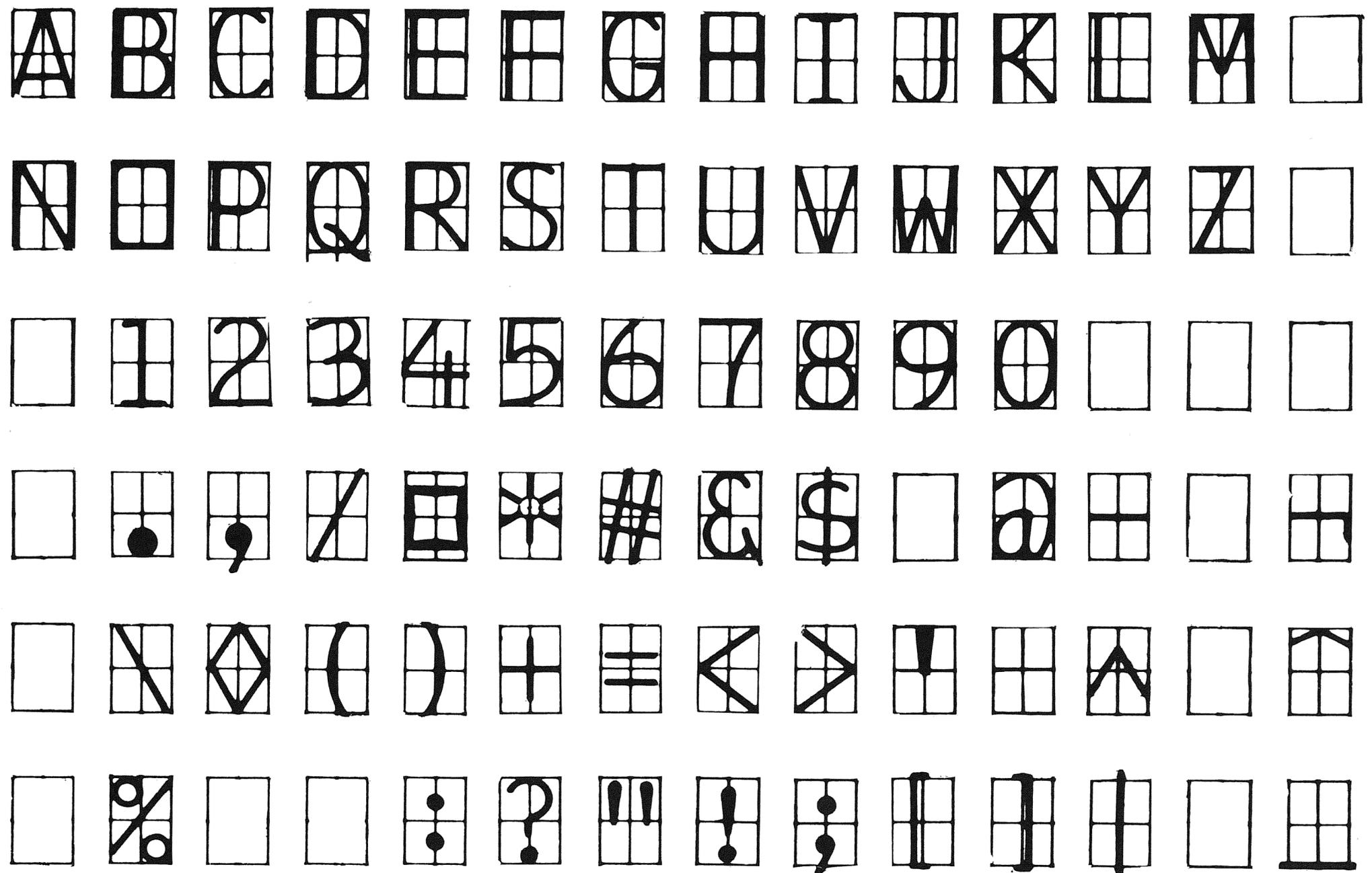
For the MDS Chain Printer (all models), the characters illustrated above are Standard Type. All alphanumeric and special graphics characters of the 16-, 48-, and 64-Character Sets of the basic standard arrangements are shown. For those characters included in a specific arrangement, see "Chain Layouts" for the appropriate printer model.
