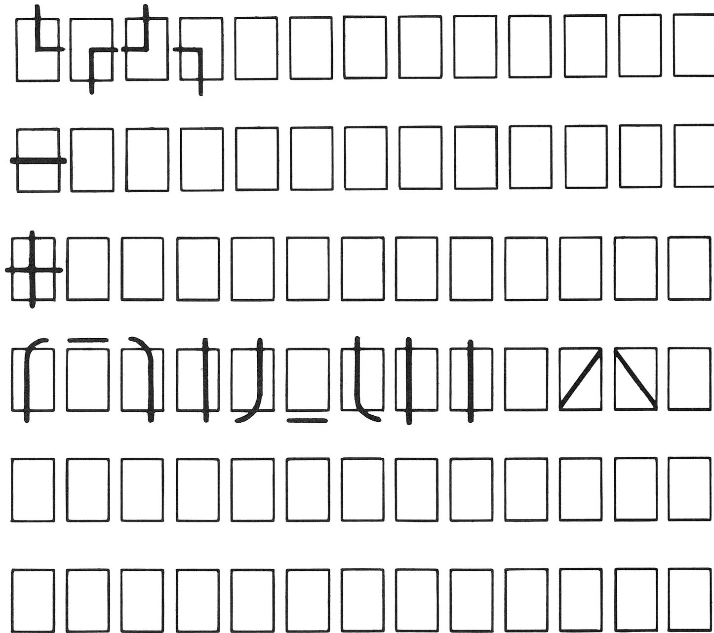
All symbols illustrated above are designed for 8 lines-per-inch spacing (vertically). Symbols shown in the upper three rows are plotting-type symbols. Symbols shown in the lower three rows are graphic segments (character strokes) for composition of large-size printout in stroke matrices.
