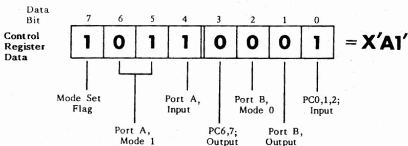
Note that PC 3,4, and 5 are used for the Port A handshaking and interrupt signals and are therefore not available for I/O ("8255A Operational Description", Figure 8); however PC 0,1,2,6, and 7 can be used for digital I/O. The interrupt signal generated on PC 3 may be jumpered to one of the the PC's interrupt channels. The interrupt channel selection was described in Chapter 2.
