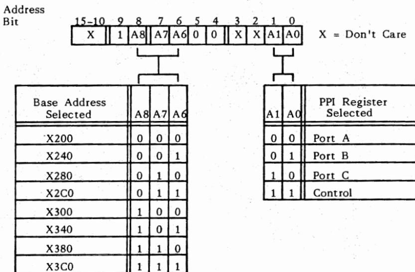
**Fig. 2-2 DG24 I/O Port Address Decode**
