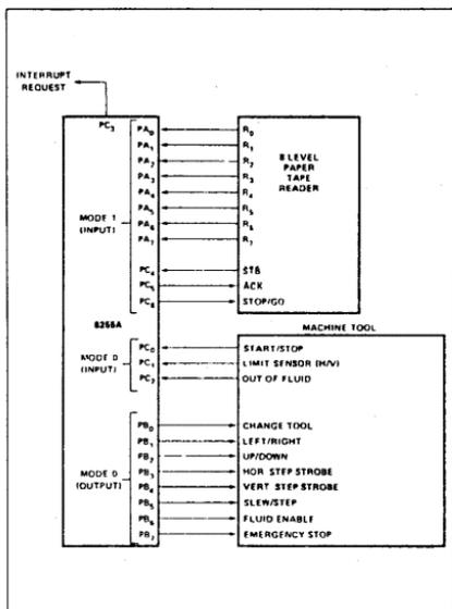
Figure 25. Machine Tool Controller Interface
