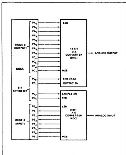
Figure 22. Digital to Analog, Analog to Digital
