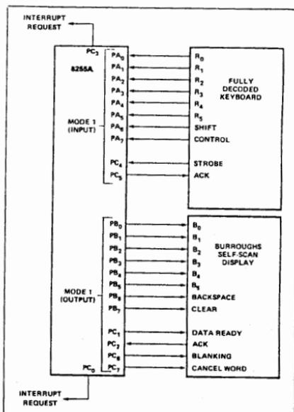
Figure 20. Keyboard and Display Interface
