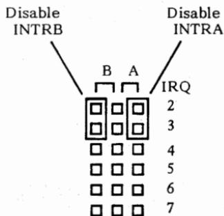
**Fig. 2-3 Interrupt Disable Jumper Positions**
