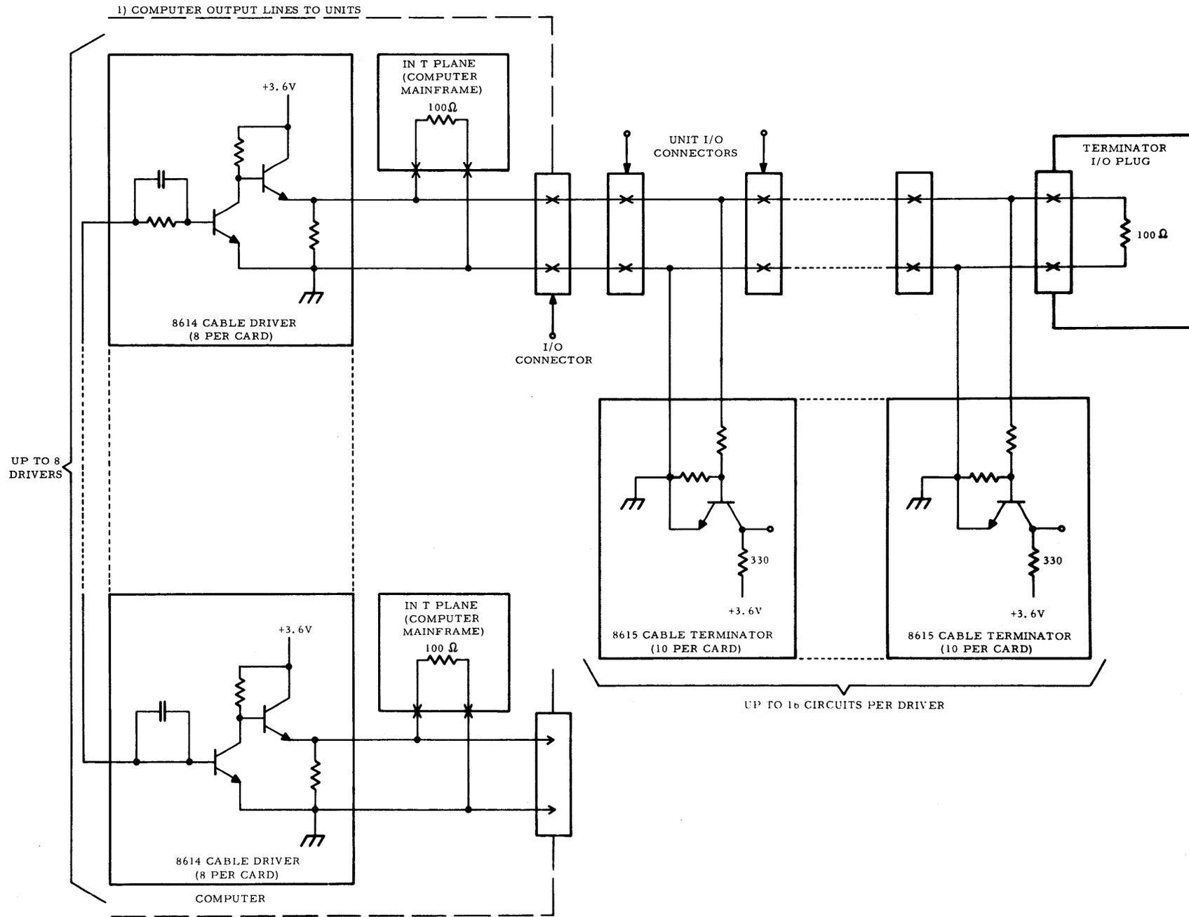
FIGURE 2.1.2-2 OUTPUT LINES FROM COMPUTER
