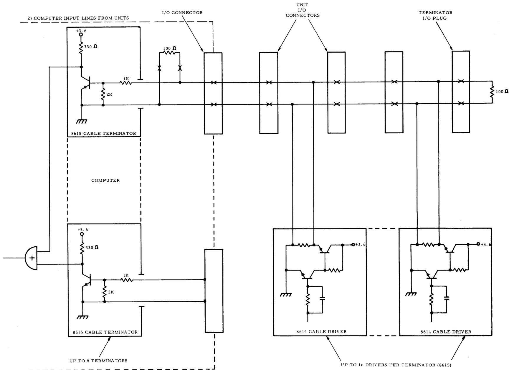
FIGURE 2.1.2-3 INPUT LINES TO COMPUTER
