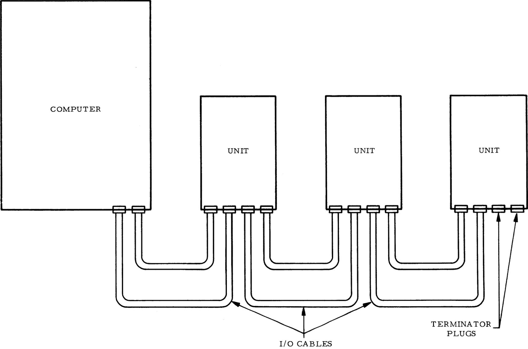
FIGURE 2.1.2-4 I/O CABLING
