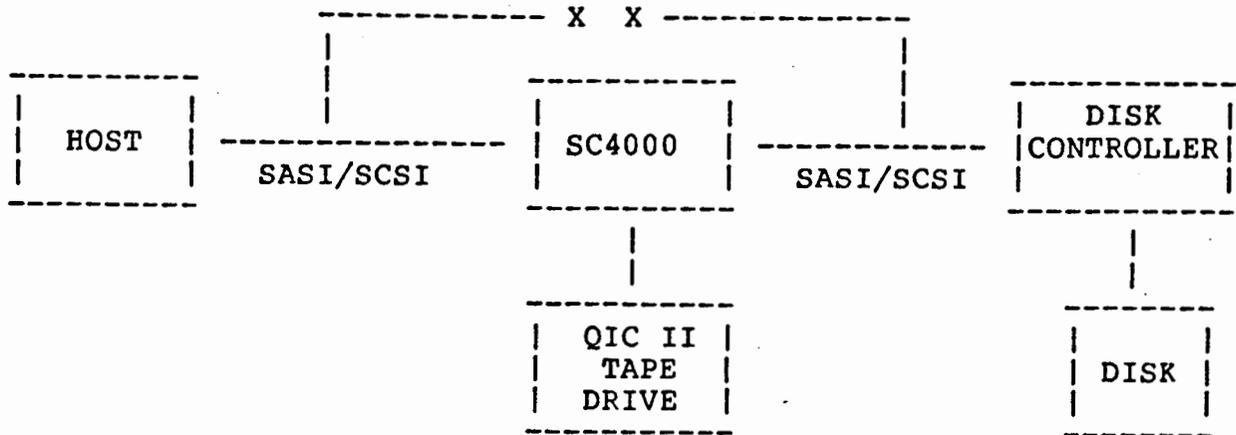
The broken path shown might have been the original system set up before installing SC4000 and QIC II tape drive.
