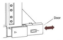
2. Grasp the door to pull the power supply out of the tunnel.
