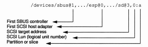
The ellipses (...) represent the virtual memory address of the corresponding device.
