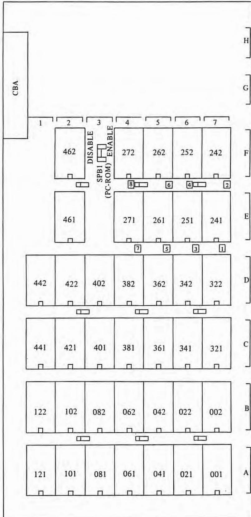
6.1.8 Connection unit (A20B-0007-0040 or A20B-0008-0540) mounting diagram
