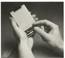
2. Replace the old batteries with new batteries. Make sure the positive (+) and negative (—) poles marked on the batteries match the poles marked in the remote control unit.
