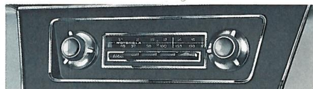
**For Buick** . . . Model BK4FM, FM/AM combination car radio blends with '64 Buick dash. Same features as FMA100 with the addition of Rear Speaker Control.
