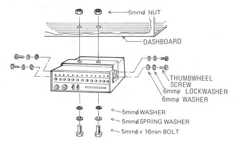
Avoid drilling in areas near wiring or other obstructions. Use Bolt and Nut to fasten bracket to dashboard. Mount the unit to the bracket with four thumbwheel screws.
