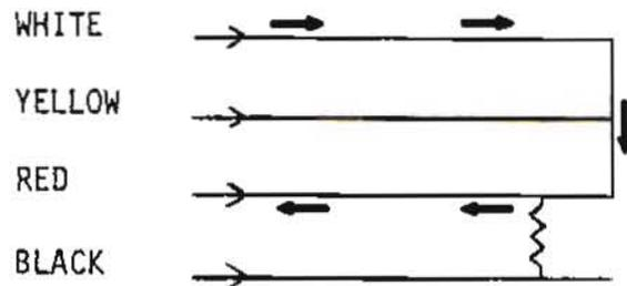
IF THE CONDUCTORS BETWEEN THE WHITE AND RED TEST LEADS ARE NOT OPEN . . . . .
