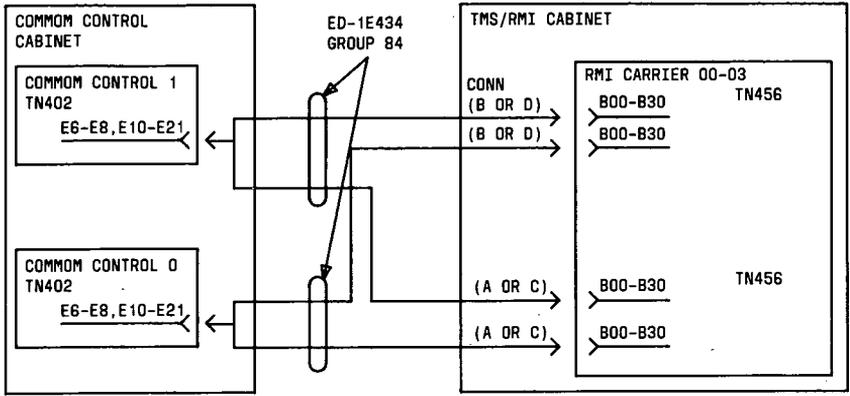
Figure 38. ED-1E434, Group 84 Connections for a Duplicated System (Phase 2)
