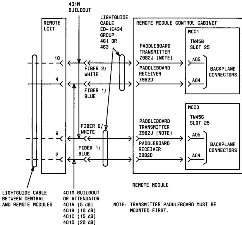
**Figure 55.** Remote RMI Fiber-Link Connections for Duplicated Module Control (Phases 1 and 2)
