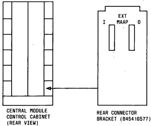
**Figure 13.** Rear Connector Plate (845416577) and Location (Phases 1 and 2)
