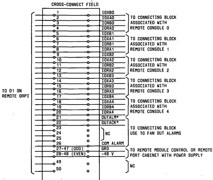
Figure 66. D1 Cross-Connect Connections
