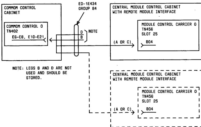
Figure 28. ED-1E434, Group 84 Connections for an All Unduplicated System (Phase 1)
