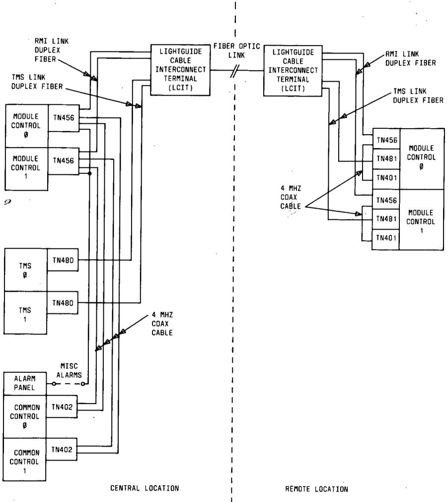
Figure 2. Duplicated RMI System (Phase 1) Block Diagram
