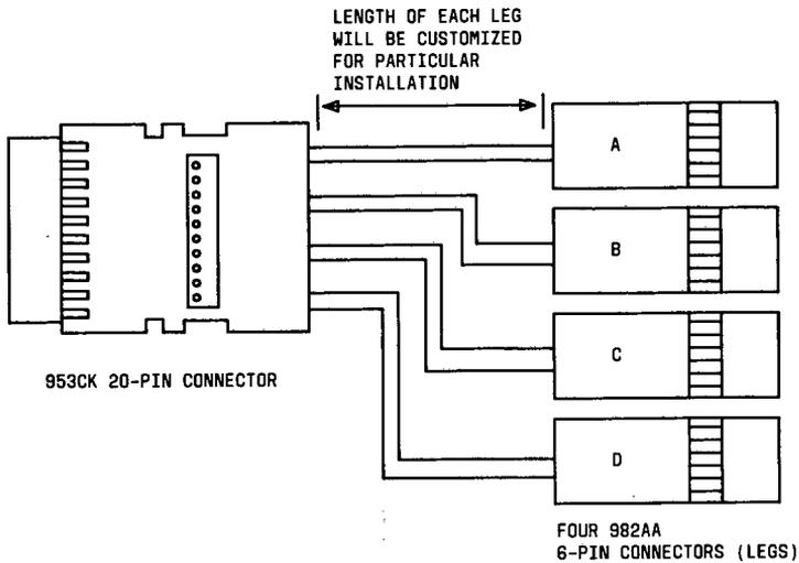
Figure 27. ED-1E434, Group 84 Coaxial Cable
