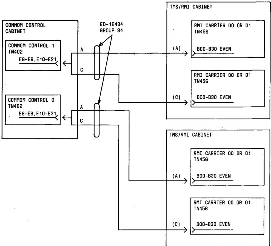
Figure 39. ED-1E434, Group 84 Connections for a Duplicated Common Control and Unduplicated Module Control System (Phase 2)
