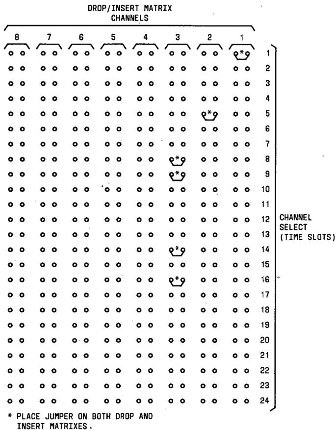
Figure 87. Drop/Insert Matrix
