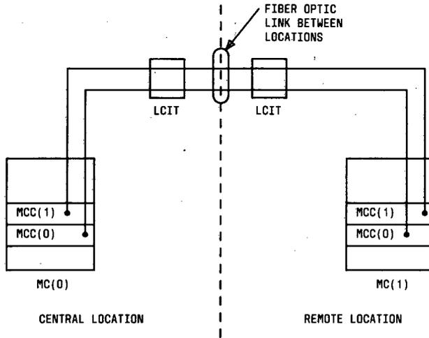
Figure 8. Assigned Module Control Carriers for a Duplicated System With One Central and One Remote Module (Phase 1)
