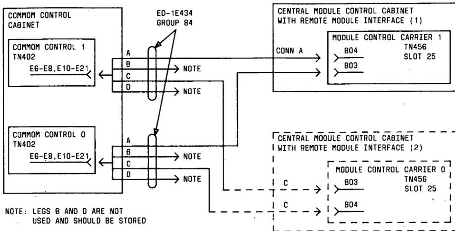
**Figure 30.** ED-1E434, Group 84 Connections for all Duplicated Common Control and Unduplicated Module Control System (Phase 1)
