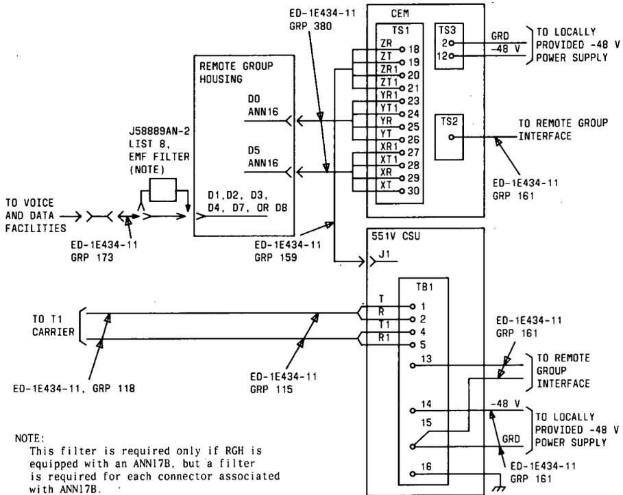
Figure 105. T1 Carrier to RGI Using CEM and CSU
