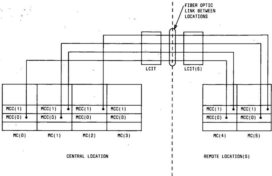
**Figure 9.** Assigned Module Control Carriers for a Duplicated System With Four Central and Two Remote Modules (Phase 1)
