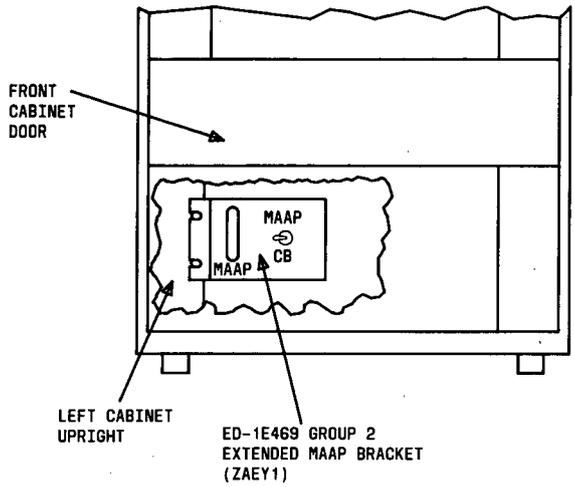
**Figure 19.** ED-1E469, Group 2 Remote Extended MAAP Bracket Mounting Location
