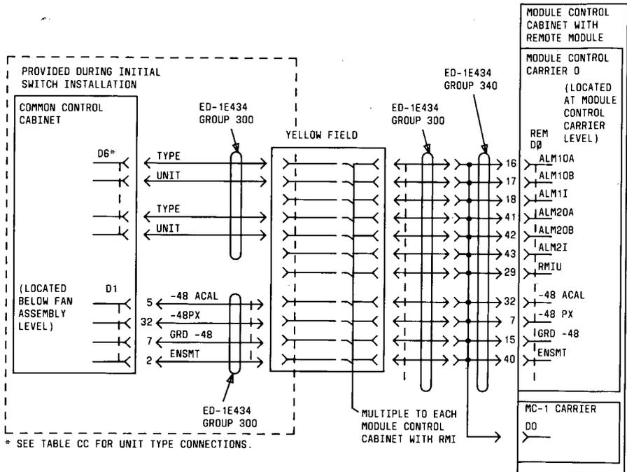
NOTE: FOR DUPLICATED SYSTEMS, AN ED-1E434 GROUP 340 CABLE IS USED TO "Y" MCO AND MC1 "DO" CONNECTORS TOGETHER, AND THEN CONNECTS TO THE GROUP CABLE.
