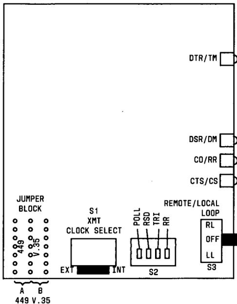
Figure 95. V.35/RS-449 Option Switch Locations
