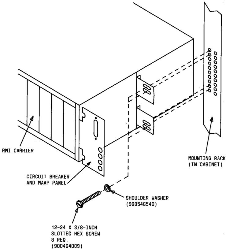
Figure 5. RMI Carrier (Phase 2) Installation
