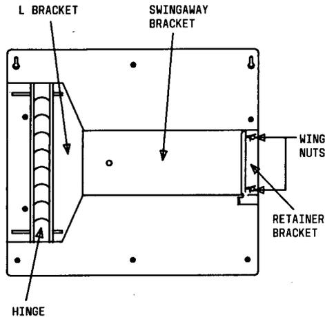
**Figure 76.** RGH Wall Mounting Bracket
