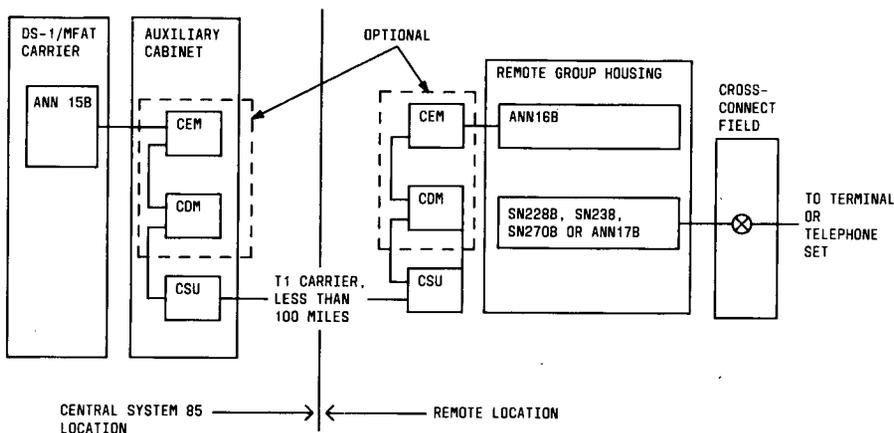
Figure 73. Remote Group Interface Block Diagram
