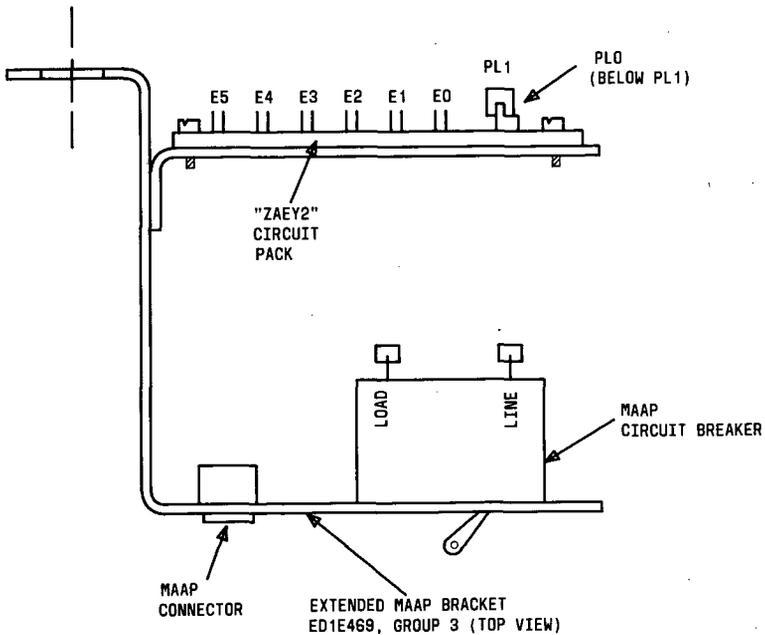
Figure 16. ED-1E469, Group 3 Central Extended MAAP Bracket (Phases 1 and 2)
