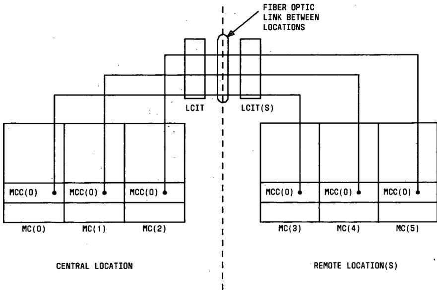
**Figure 7.** Assigned Module Control Carriers for Unduplicated System (Phase 1)
