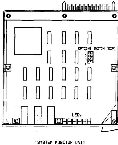
**Figure 84.** System Monitor Unit
