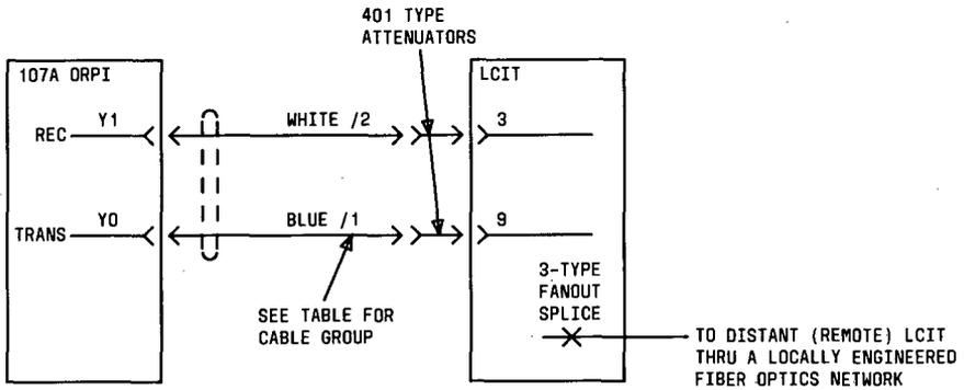
**Figure 64. ORPI to LCIT Connections**
