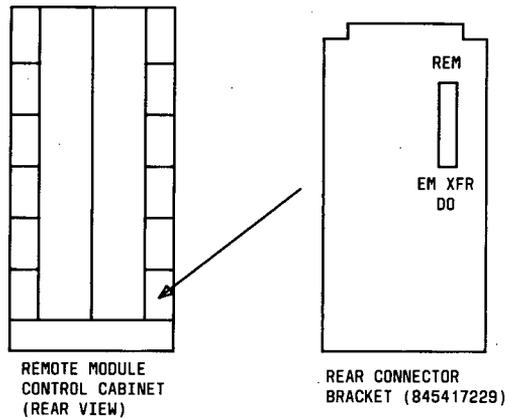
**Figure 14.** Rear Connector Plate (845417229) and Location (Phases 1 and 2)
