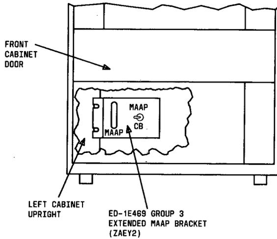
**Figure 17.** ED-1E469, Group 3 Central Extended MAAP Bracket Mounting Location
