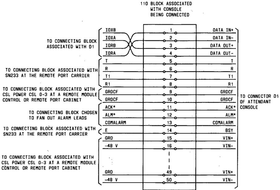
Figure 68. Console Connector Terminating Information
