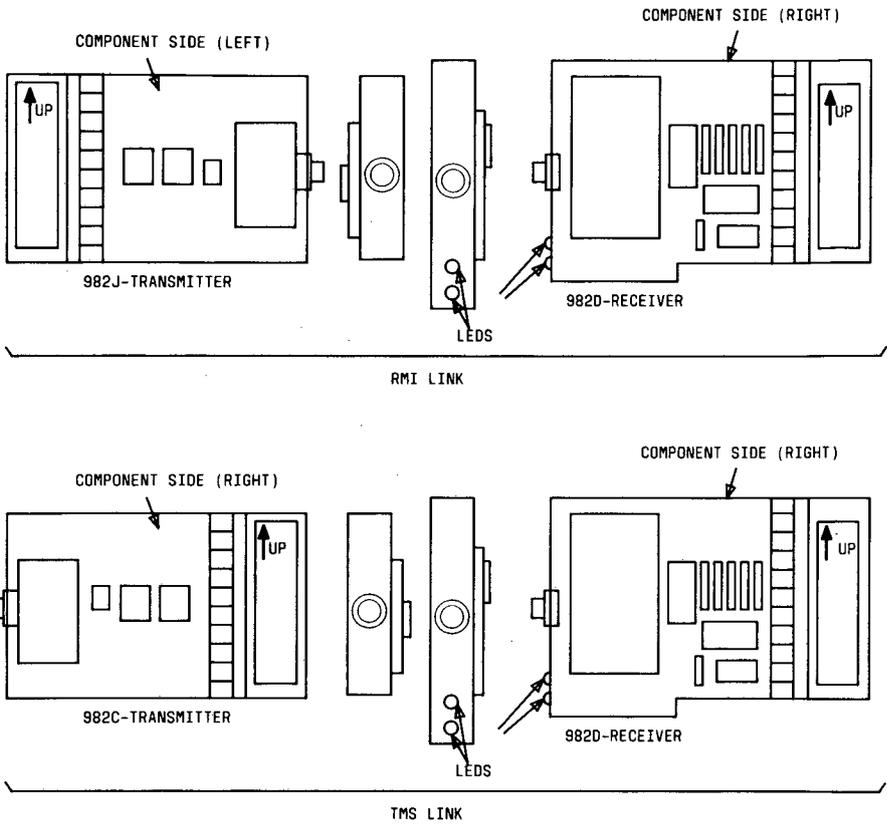
Figure 45. Z982J, Z982C, and Z982D Paddleboards and Mounting Locations.
