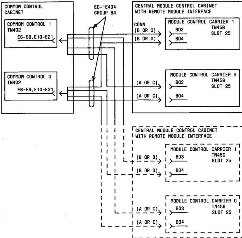
Figure 29. ED-1E434, Group 84 Connections for an All Duplicated System (Phase 1)
