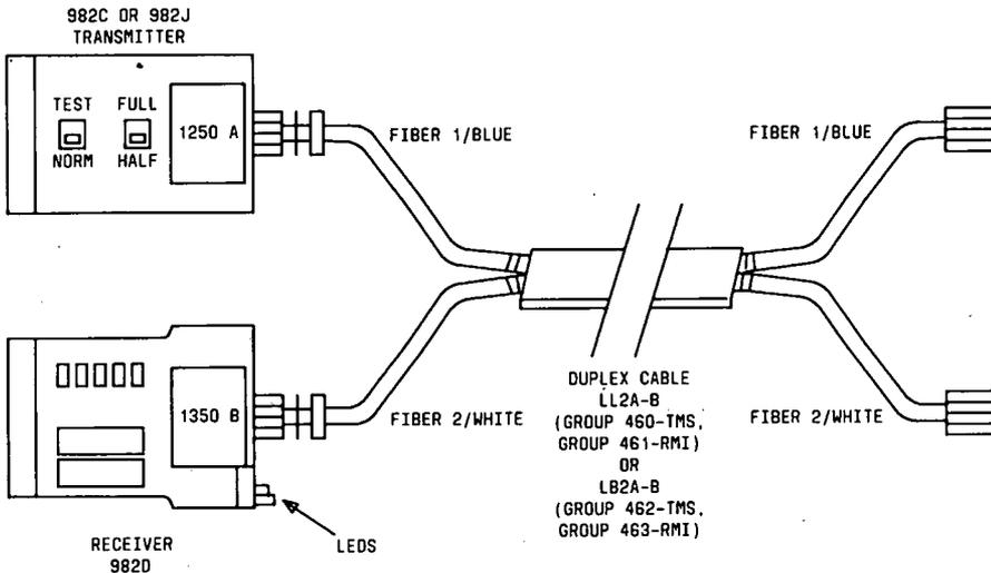
Figure 44. Duplex Cable (Lightguide) With Paddleboard Transmitter and Receiver
