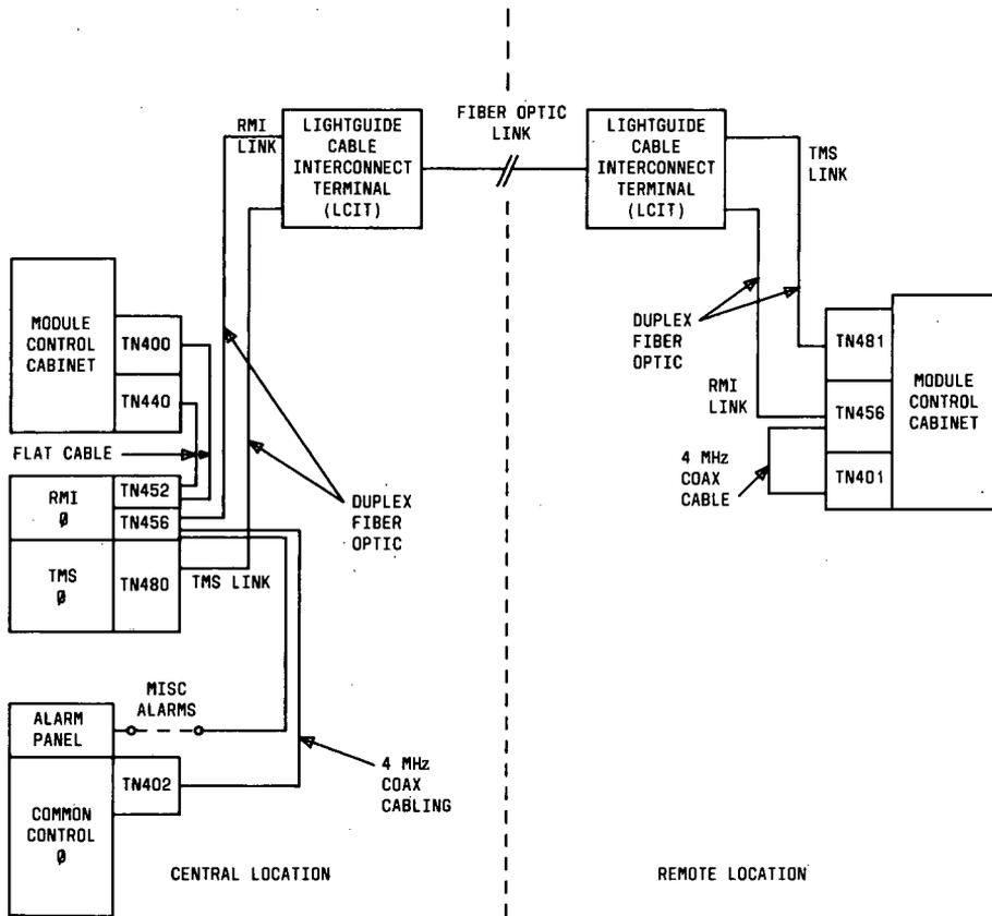
Figure 3. Unduplicated RMI System (Phase 2) Block Diagram
