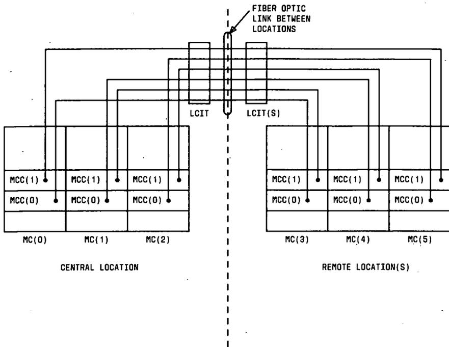
**Figure 10.** Assigned Module Control Carriers for a Duplicated System With Three Central and Three Remote Modules (Phase 1)
