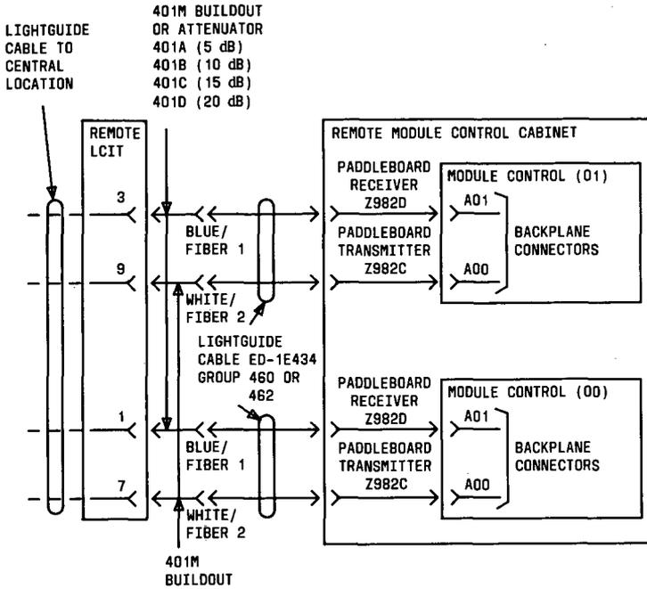
Figure 57. Remote TMS Fiber-Link Connections for Duplicated Module Control (Phases 1 and 2)
