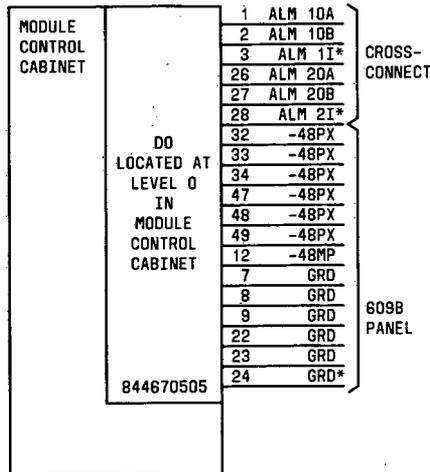
\* ONLY 2 ALARMS CAN BE ACTIVATED FOR EXTERNAL EQUIPMENT, ALM1I AND ALM2I. THERE MUST ALSO BE A GROUND LEAD FOR -48V FROM PIN 24.
