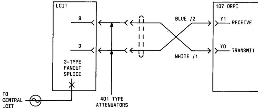
**Figure 65.** ORPI to LCIT Connections
