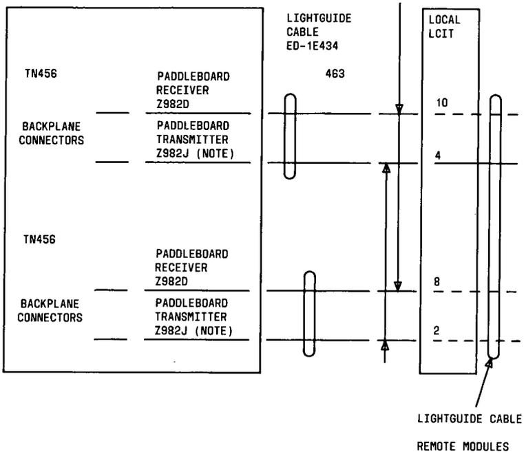
Figure 51. Central RMI Fiber-Link Connections for Duplicated Module Control (Phase 2)
