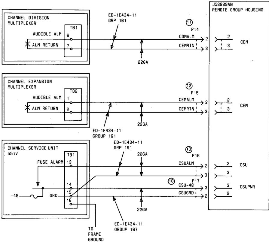
Figure 101. CSU, CDM, and CEM Power, Grounding, and Alarms
