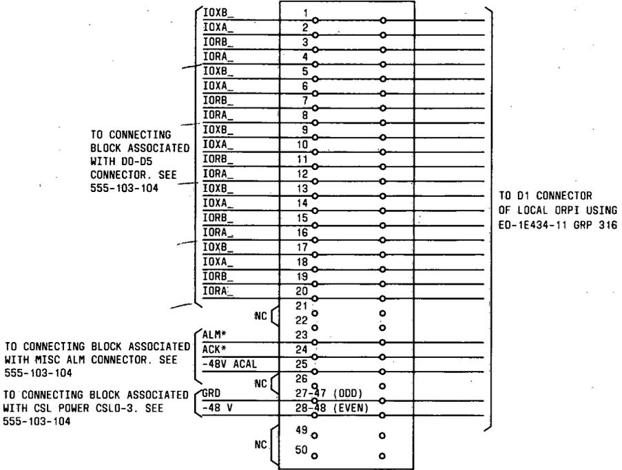
Figure 63. System 85 to ORPI Connections
