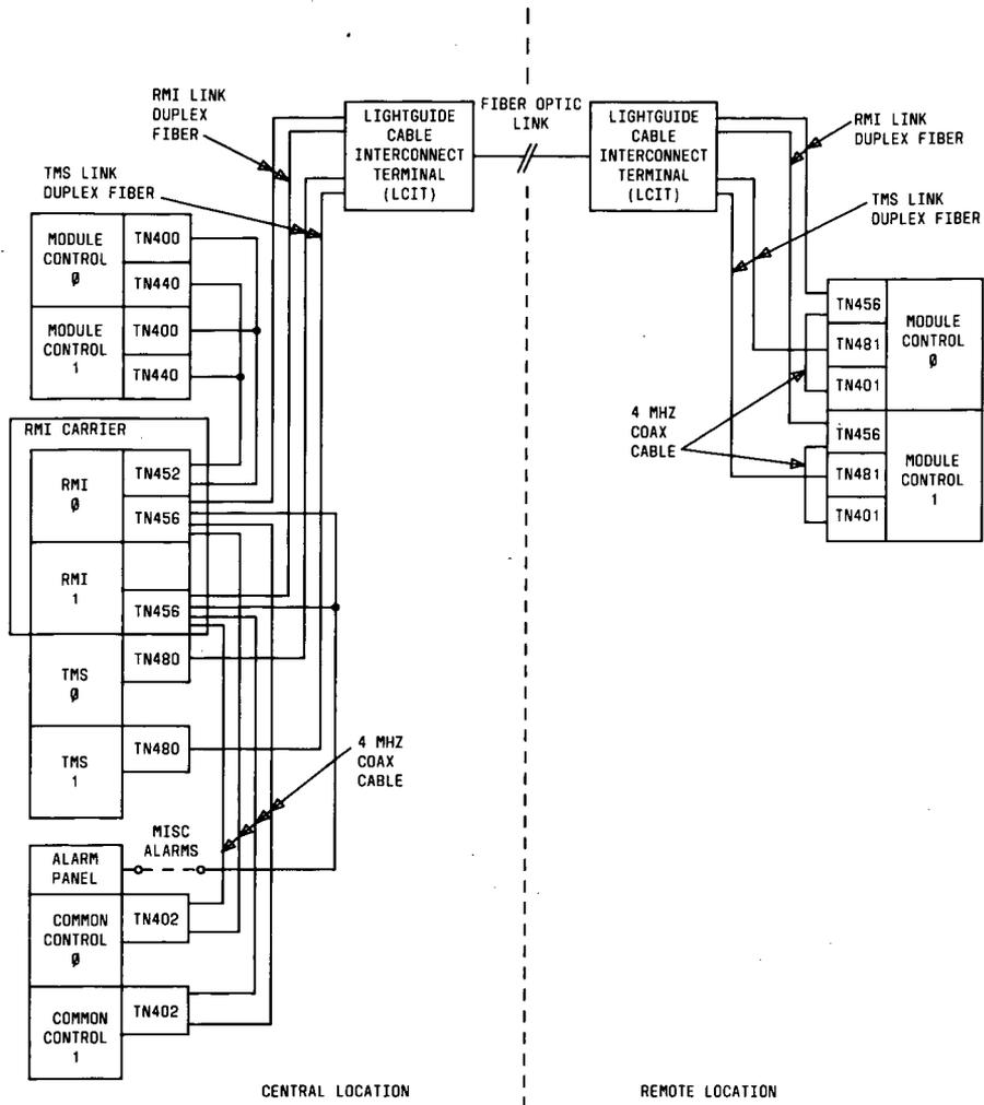
Figure 4. Duplicated RMI System (Phase 2) Block Diagram
