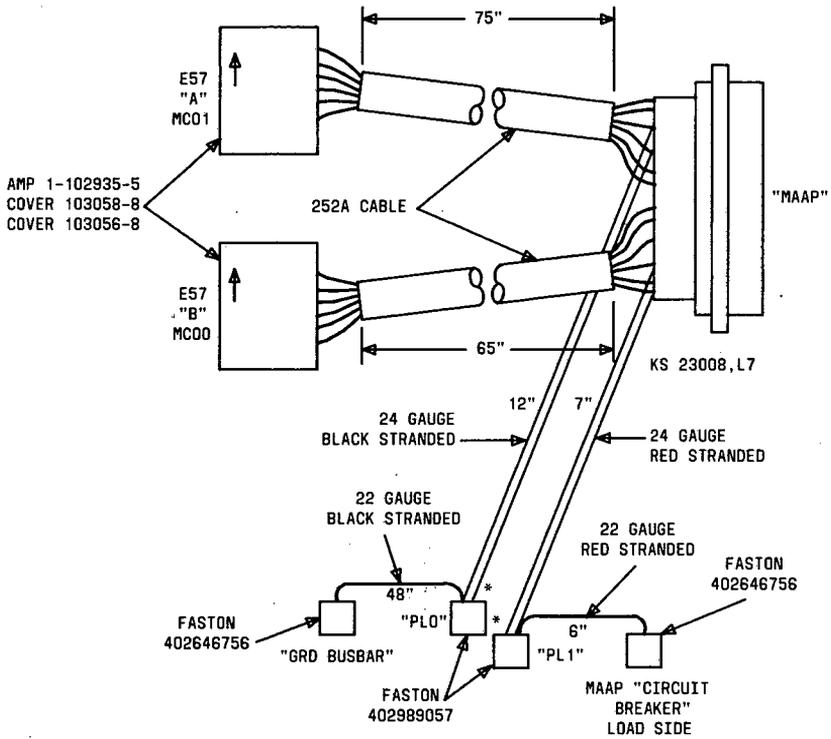
\* INSULATE WITH HEAT SHRINK TUBING
