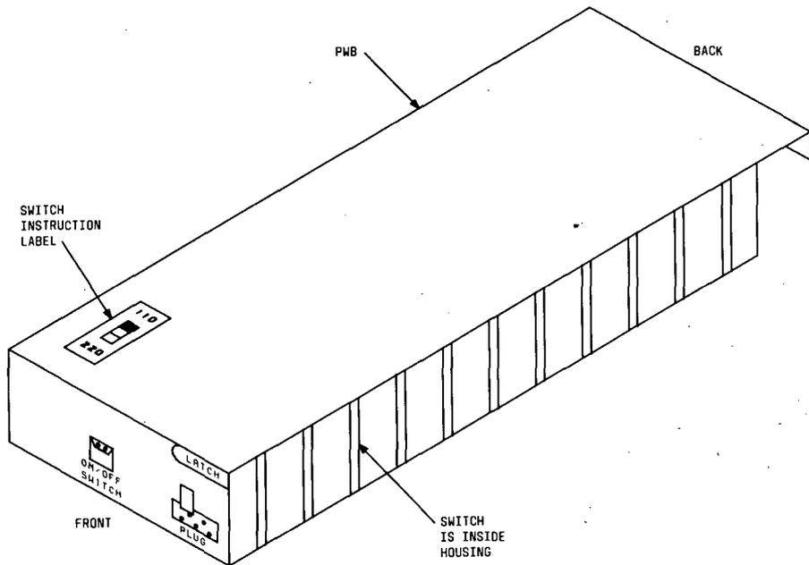
Figure 83. 634WAAB1 Switch Locations
