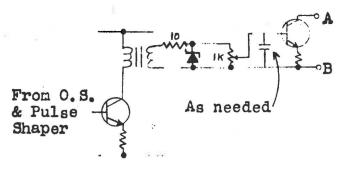
This circuit has the advantage that it can pass a constant current from either the positive or negative voltages. For positive, A goes to a positive voltage and B is the output. For negative, B goes to a negative and A is the output. Any number can be connected to the same output terminal.
