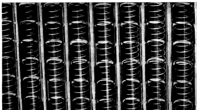
Fig. 10—Detailed structure of the grid. The exterior electrodes are pieces of metal foil cemented to the outside of the tube. The interior electrode is a long spiral of wire.
