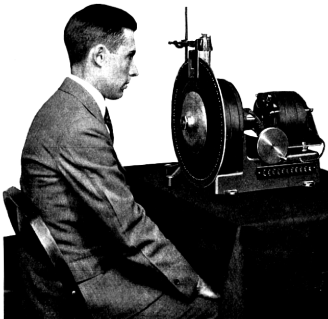
Fig. 6—Illustrative receiving apparatus. A neon lamp operated from the picture current illuminates a series of small apertures as they pass across the field of view; the observer sees an image reproduced in the frame.
