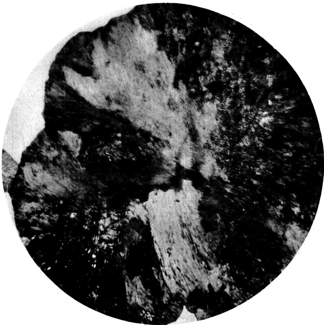
Fig. 6—Mag. 3500X. Fig. 6 is of a larger nodule than illustrated in Fig. 5 and shows obviously a little later stage in the process of stratification. This nodule is about the same as the one illustrated in Fig. 1 except that the structure has been resolved.
