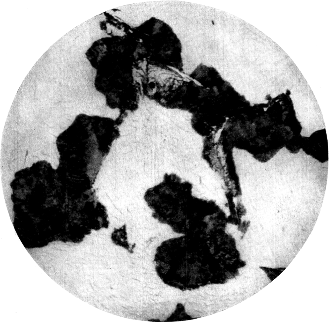
Fig. 4—Mag. 3500X. * Fig. 4 shows a somewhat later period in development of troostite. The troostite appears to have formed along grain boundaries. The excess constituent is clearly seen, and here and there a laminated structure, pearlite. Evidently whatever the state of the carbide with reference to the iron in troostite—whether contained in solid solution as first formed or whether disposed as a fine aggregate with the iron—the condition must be very unstable, otherwise evidences of finely laminated pearlite would be lacking.
