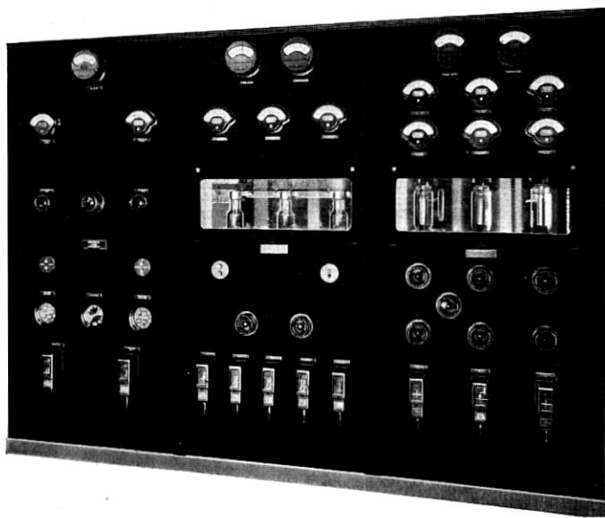
Fig. 5—Power panel and rectifier assembly for 50-kw radio transmitter.
