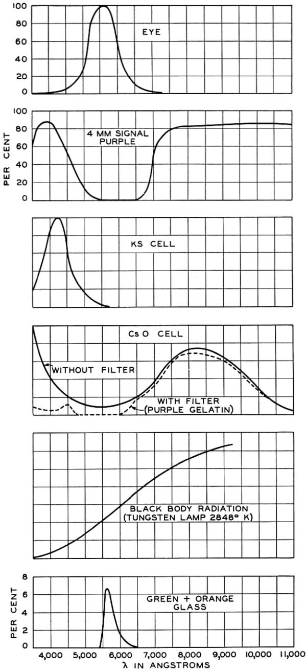
Fig. 3—Spectral characteristics of the scanning, viewing and illumination elements in two-way television system.
