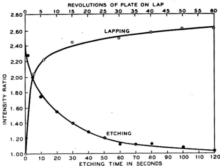
Fig. 3.—Effect on reflection-intensity produced by lapping on etched plate with 303½ emery and soap solution and by etching the lapped plate with 48% hydrofluoric acid at 25°C.
