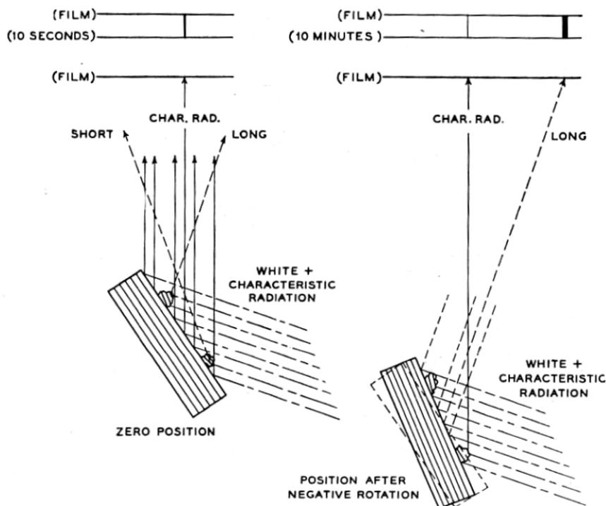
Fig. 4.—Spectrometer photography of misoriented crystalline material
