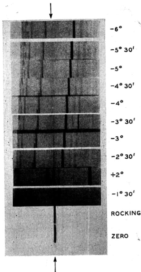
Fig. 5.—Spectrometer photograph of BT quartz plate lapped with 303½ emery
