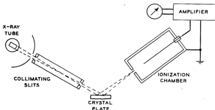
Fig. 2.—Single crystal spectrometer
