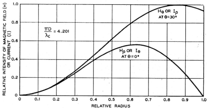
Fig. 8—End plate currents in TE 31 mode.
