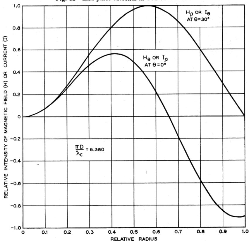
Fig. 13—End plate currents in TM 31 mode.
