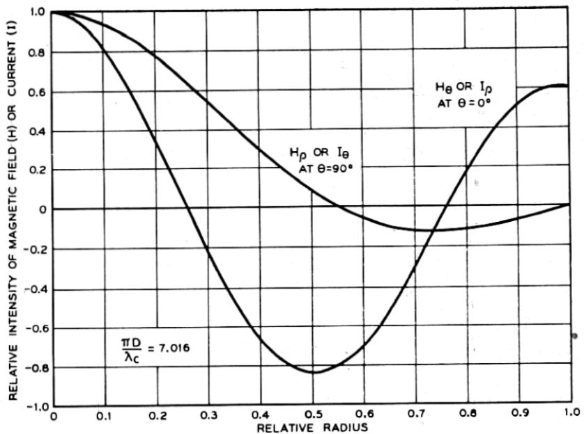
Fig. 16—End plate currents in TM 12 mode.
