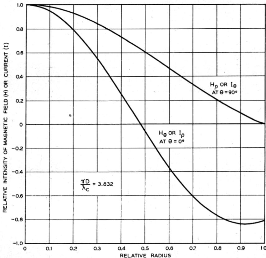
Fig. 6—End plate currents in TM 11 mode.
