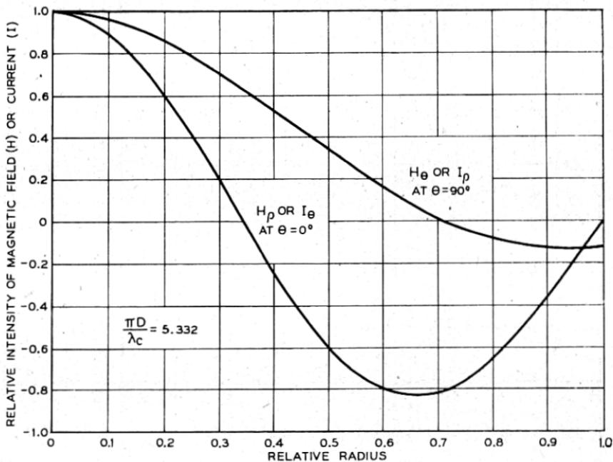
Fig. 11—End plate currents in TE 12 mode.
