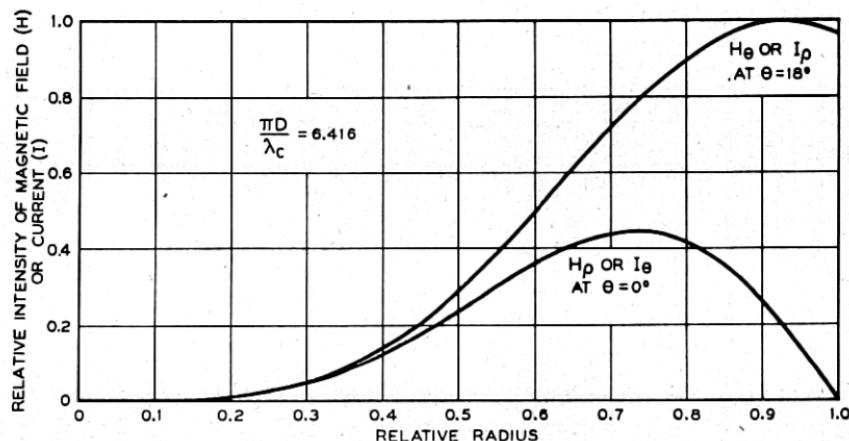
Fig. 14—End plate currents in TE 51 mode.
