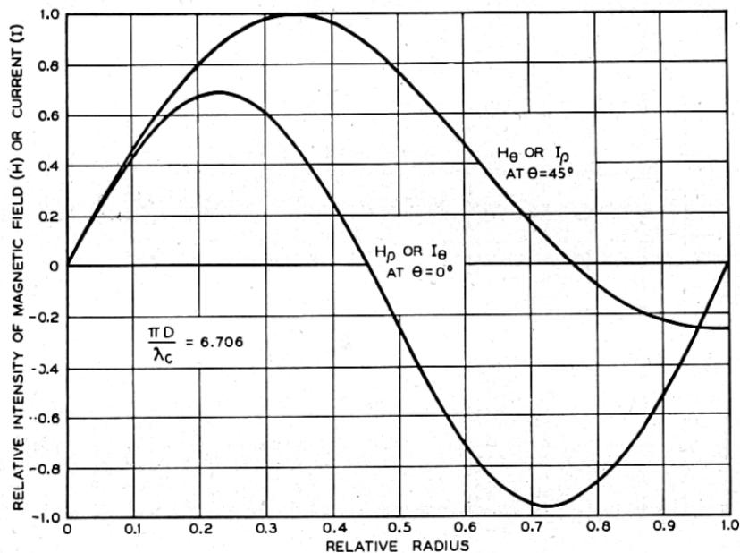
Fig. 15—End plate currents in TE 22 mode.
