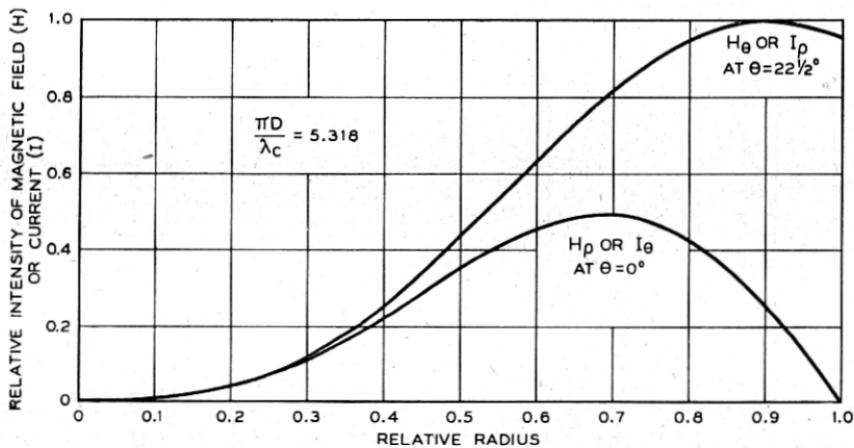
Fig. 10—End plate currents in TE 41 mode.
