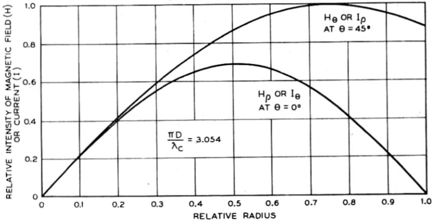
Fig. 5—End plate currents in TE 21 mode.
