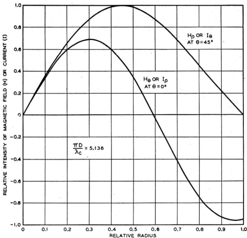
Fig. 9—End plate currents in TM 21 mode.
