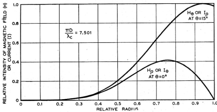
Fig. 18—End plate currents in TE 61 mode.
