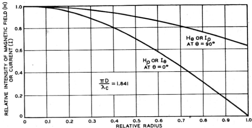
Fig. 3—End plate currents in TE 11 mode.
