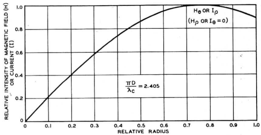
Fig. 4—End plate currents in TM 01 mode.
