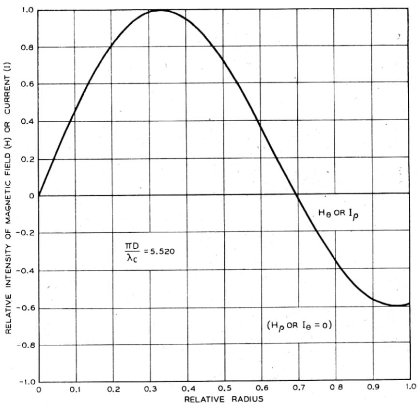
Fig. 12—End plate currents in TM 02 mode.
