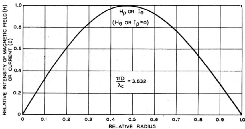
Fig. 7—End plate currents in TE 01 mode.
