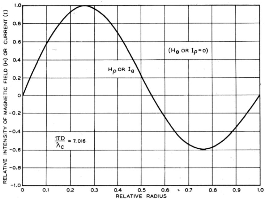
Fig. 17—End plate currents in TE 02 mode.
