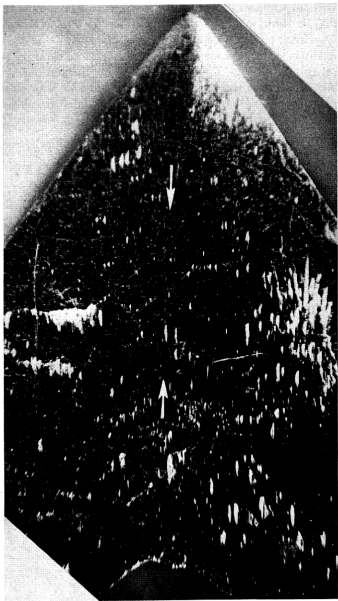
Fig. 4 — Picture of domain pattern at one corner of sample. The stationary wall is indicated by arrows.
