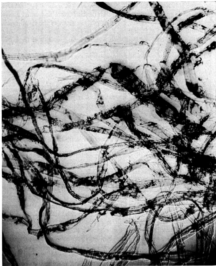
FIG. 13 — Paper fibers removed from cathodic area showing dendritic silver deposits.
