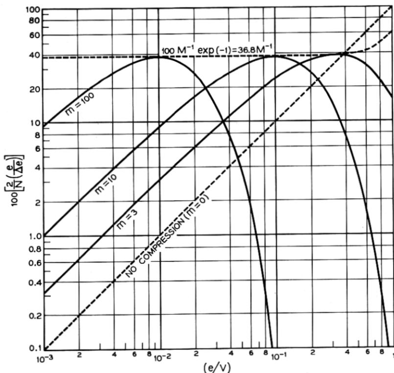
Fig. 23 — Pulse sample to step size ratios as a function of relative sample amplitude, for various companders in the  $m$ -ensemble. The maxima exhibited by these curves occur at  $e/V = m^{-1}$ ;  $M = 1 - \exp(-m)$ . Compare with Fig. 5.
