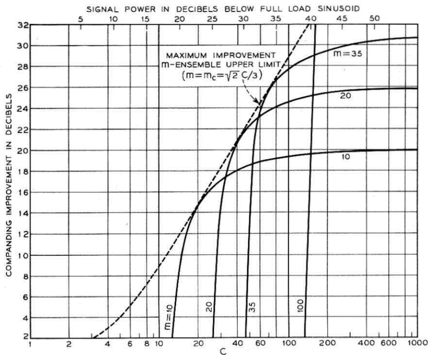
Fig. 25 — Companding improvement curves for representative members of the  $m$ -ensemble. These curves are to be compared with those for the  $\mu$ -ensemble in Fig. 8. Note the important difference between the two ensembles for strong signals (small values of  $C$ ).
