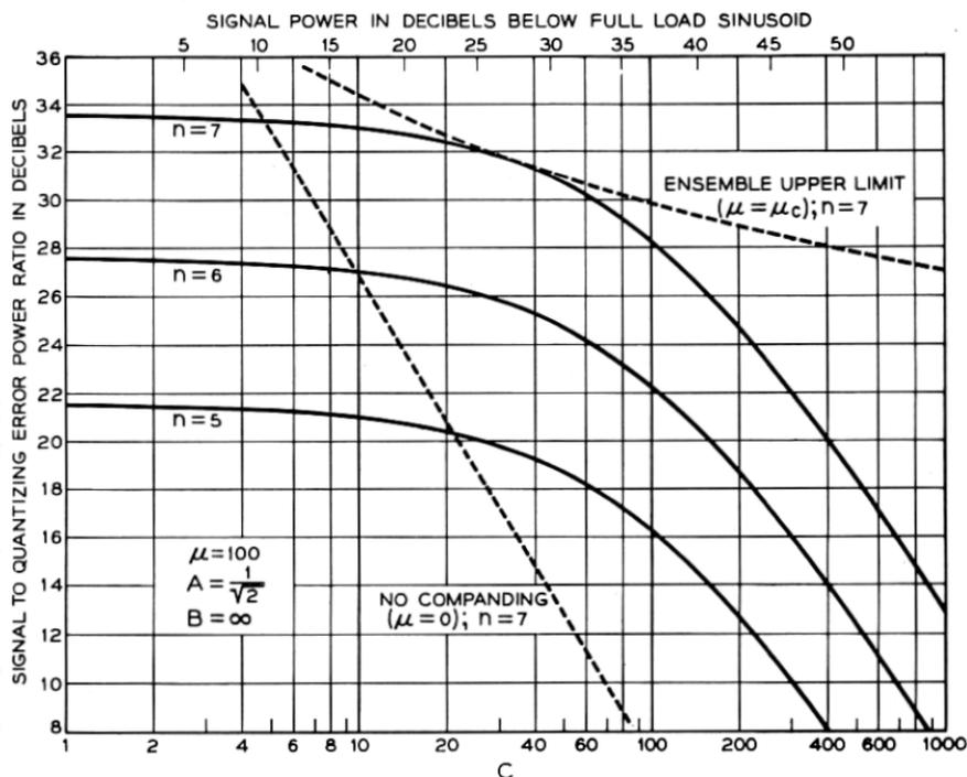
Fig. 15 — Signal to quantizing error power ratios (calculated, in db, from equation (39)) as a function of relative signal power for companding corresponding to  $\mu = 100$ . Curves are shown for  $n = 5, 6,$  and  $7$  digits per code group. For comparison, the results for seven digits in the absence of companding ( $\mu = 0$ ) as well as for the ensemble upper limit ( $\mu = \mu_c$ ) are included.  $B = \infty$  throughout.
