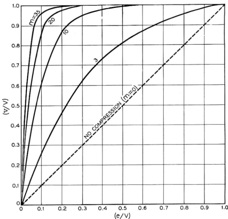
Fig. 21 — Typical  $m$ -ensemble compression characteristics determined by equation (A-7). Note the strong emphasis on weak signal amplitudes. These curves may be compared with those for the  $\mu$ -ensemble in Fig. 3.
