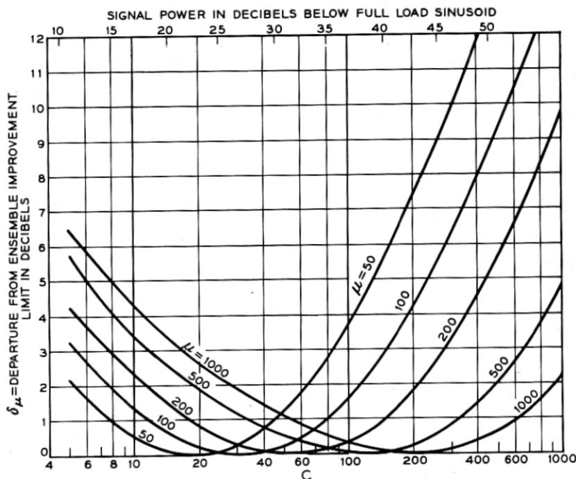
Fig. 14 — Improvement selectivity, i.e., departures from the ensemble upper limit of improvement due to the use of a single value of  $\mu$  rather than the ensemble of  $\mu_c$  values. The minima at  $\delta_\mu = 0$  locate the signals ( $C$ ) for which  $\mu$  and  $\mu_c$  coincide. All curves correspond to the case where the "dc component",  $e_0$ , is zero.
