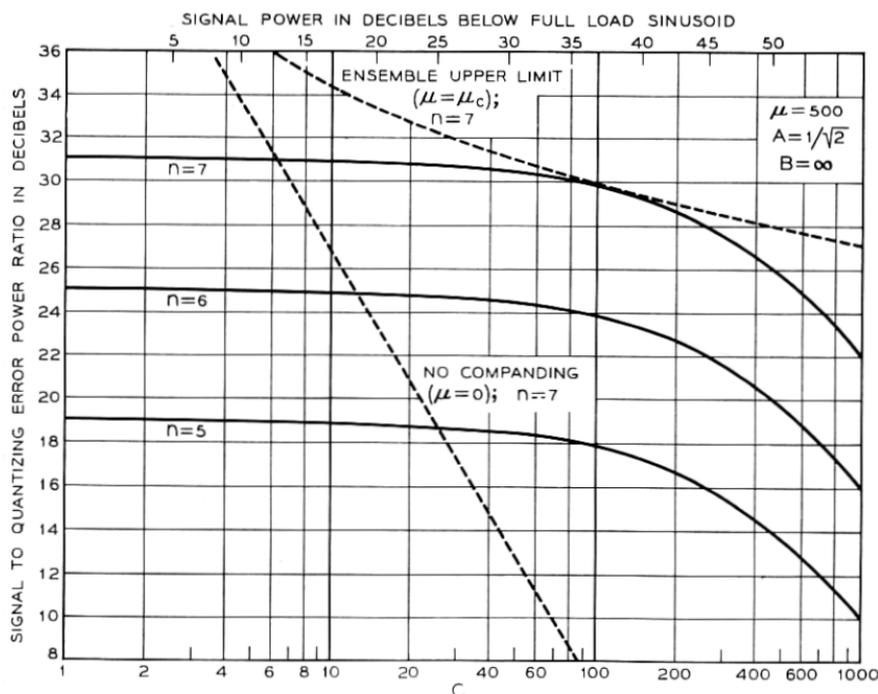
Fig. 17 — Signal to quantizing error power ratios (in db) as a function of relative signal power for companding corresponding to  $\mu = 500$ . Symbols have the same significance as in Fig. 15.  $B = \infty$  throughout.
