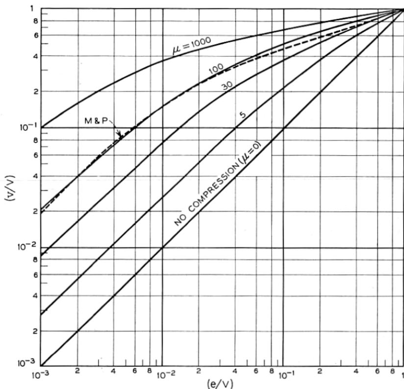
Fig. 4 — Logarithmic replot of compression curves shown in Fig. 3, to indicate detailed behavior for weak samples. The characteristic employed in the experiments of Meacham and Peterson<sup>6</sup> (M & P) is also shown. Similarity between this characteristic and the  $\mu = 100$  curve testifies to the probable realizability of these logarithmic characteristics.
