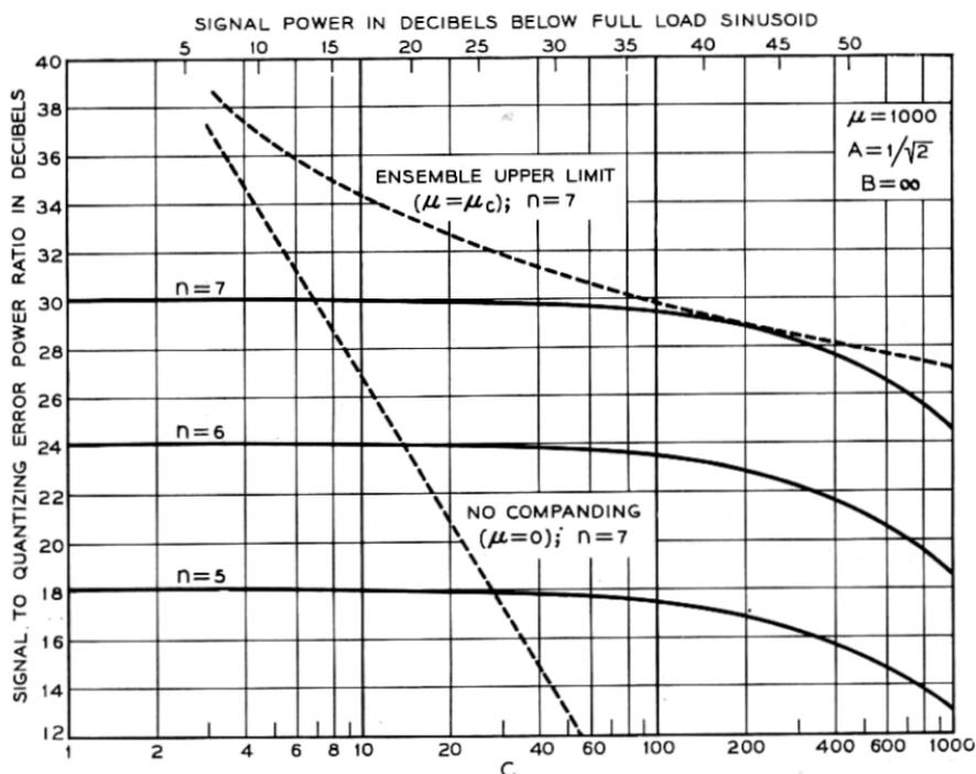
Fig. 18 — Signal to quantizing error power ratios (in db) as a function of relative signal power for companding corresponding to  $\mu = 1,000$ . Symbols have the same significance as in Fig. 15.  $B = \infty$  throughout.
