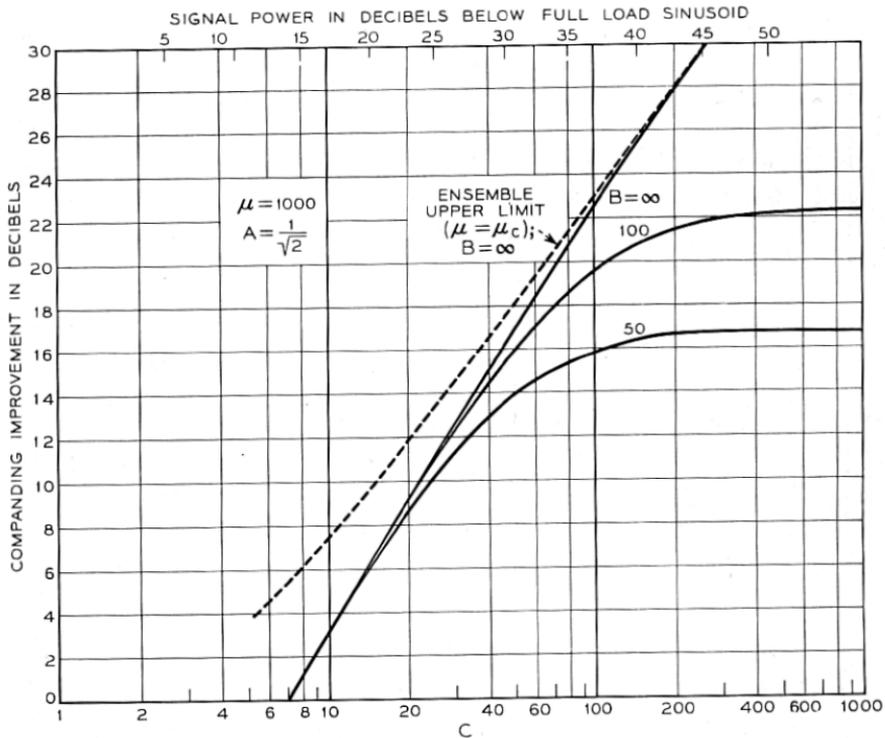
Fig. 13 — The effect of a "dc component" on companding improvement for  $\mu = 1,000$ . For further details, see the caption of Fig. 10.
