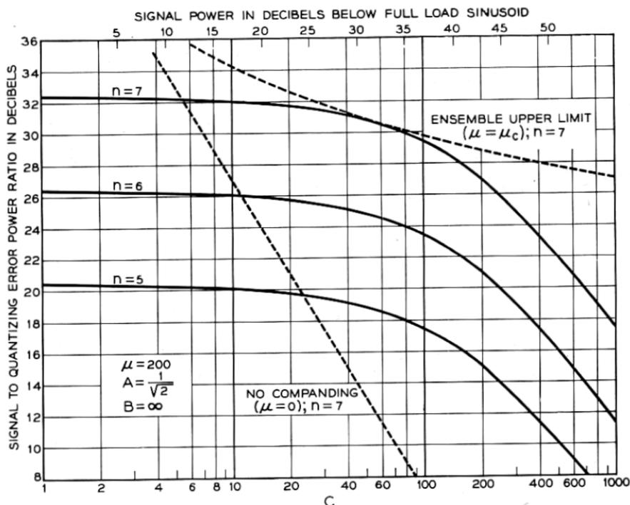
Fig. 16 — Signal to quantizing error power ratios (in db) as a function of relative signal power for companding corresponding to  $\mu = 200$ . Symbols have the same significance as in Fig. 15.  $B = \infty$  throughout.
