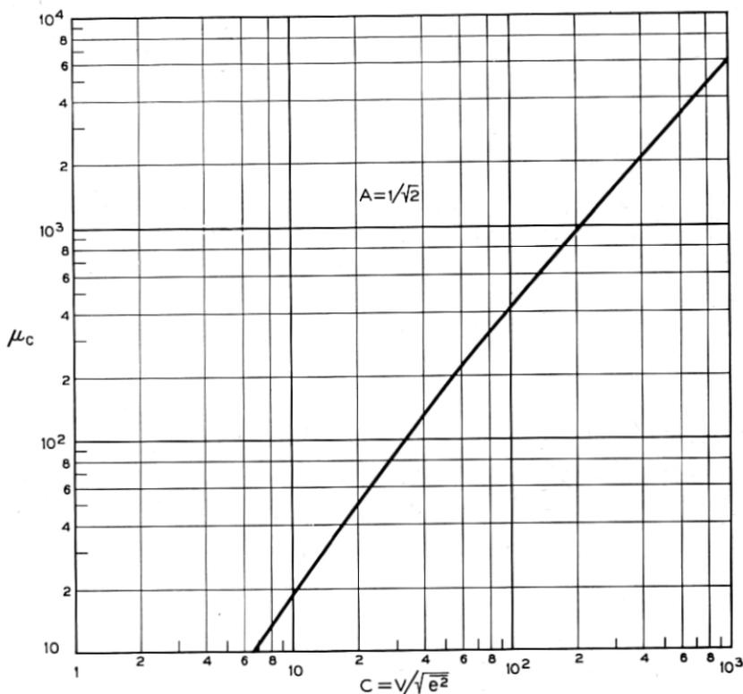
Fig. 7 — Critical compression parameters,  $\mu_c$ , required to minimize the quantizing error power as a function of relative signal strength, as determined by equation (36). Each point on the curve defines a compander in the optimum compander ensemble. It must be understood that such an ensemble provides the best performance consistent with equation (8) rather than the absolute minimum quantizing error discussed in the Appendix.
