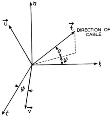
Fig. 27 — Definition of the spherical polar coordinates  $\theta$  and  $\psi$  and the unit vectors  $\vec{i}$ ,  $\vec{u}$ , and  $\vec{v}$ .
