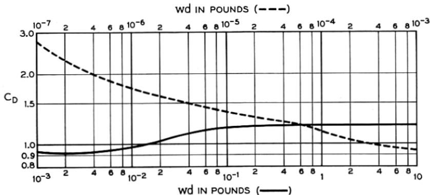
Fig. 31 — Variation of  $C_D$  with  $wd$  for cables of smooth exterior.
