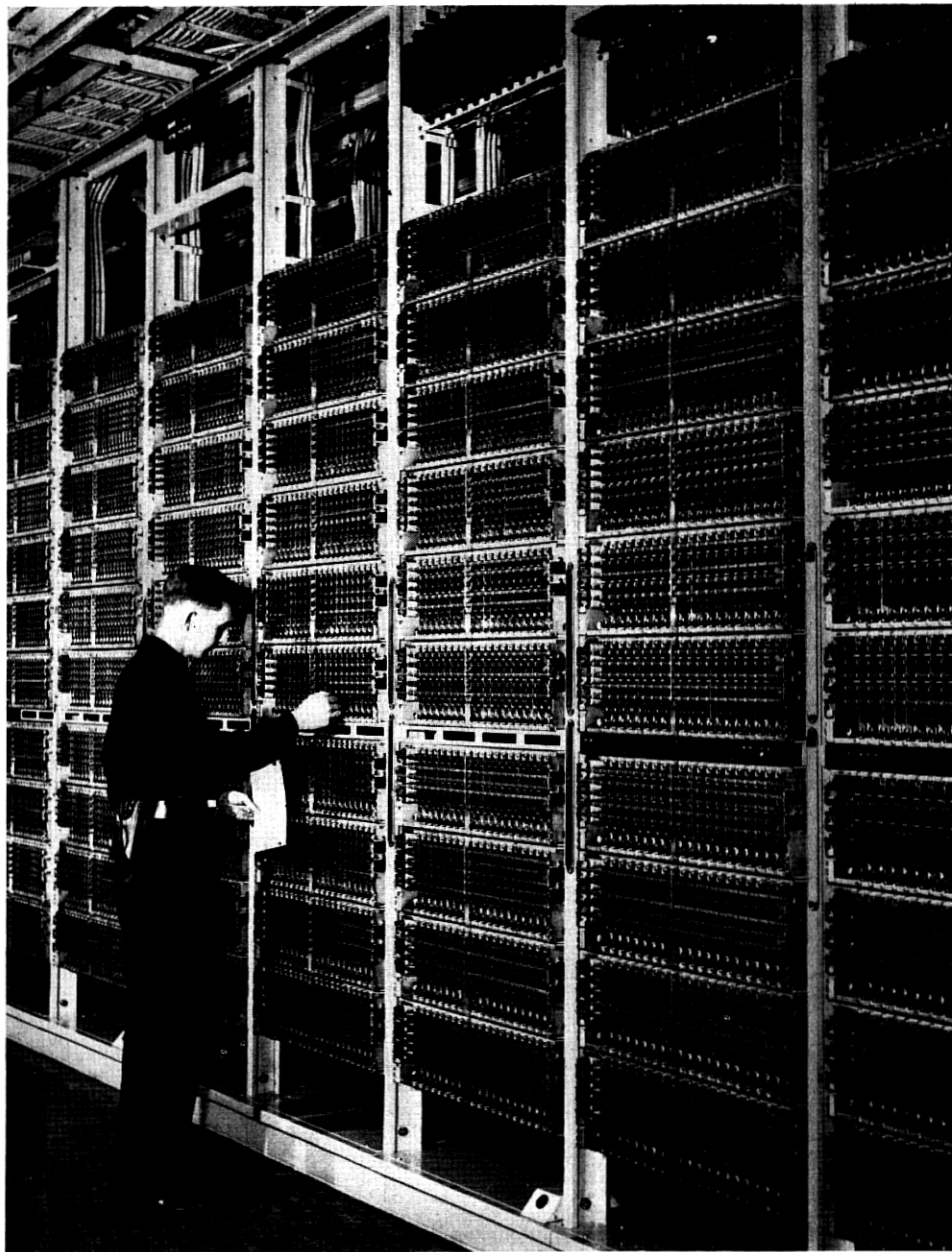
Fig. 18 — Part of a crossbar switching system.
