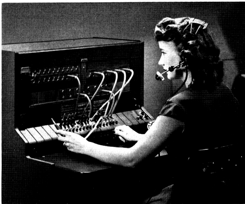
Fig. 20 — Private branch exchange switchboard, capable of handling both internal and central office calls. Used in business offices.
