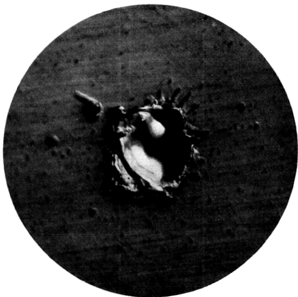
Fig. 4 — Pit made on the anode by a single arc of the anode type.
