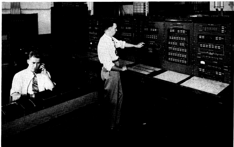
Fig. 6 — Circuit control board and main receiving station for appraisal tests.
