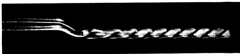
Fig. 8 — Twin-wire terminal of wire-spring relay.
