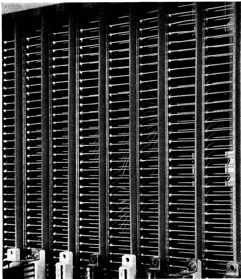
Fig. 10 — Junctor wiring at rear of connectors for central stage switches.
