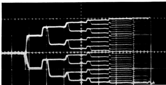
Fig. 23 — Performance of the feedback network. Each trace of the oscilloscope represents one of the 128 possible combinations of the network resistors. The lowest trace occurs when all of the network resistors are sequentially connected to \xi , the reference voltage. The highest trace occurs when all network resistors are sequentially connected to ground.
