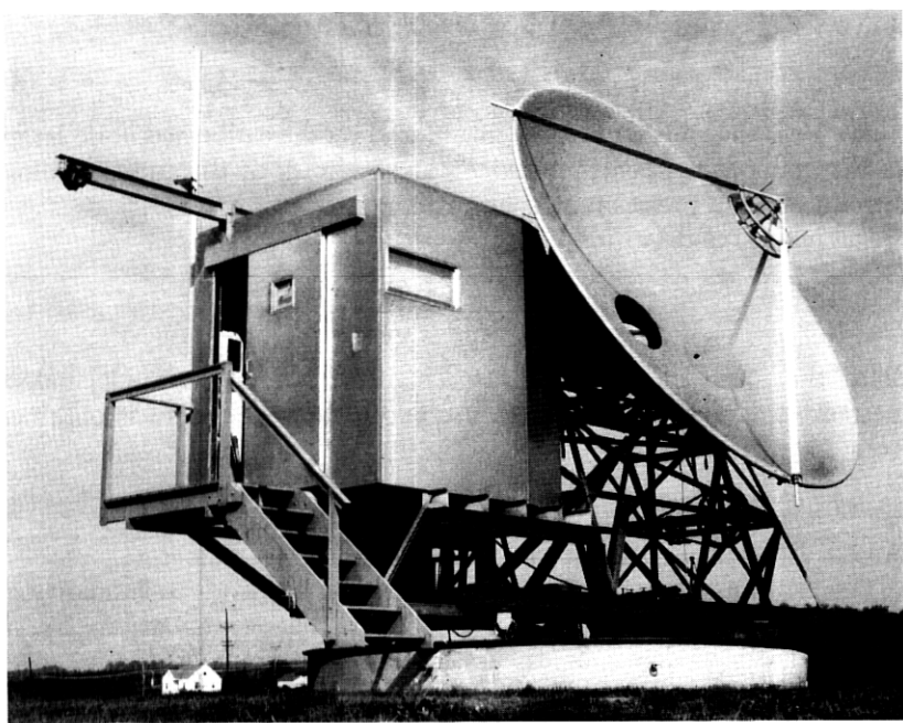
Fig. 5 — A 16-foot diameter paraboloid ( f/D = 0.375 ) with near-field Cassegrainian feed.
