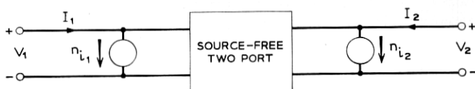
Fig. 3—Separation of twoport with internal noise sources into a source-free twoport.
