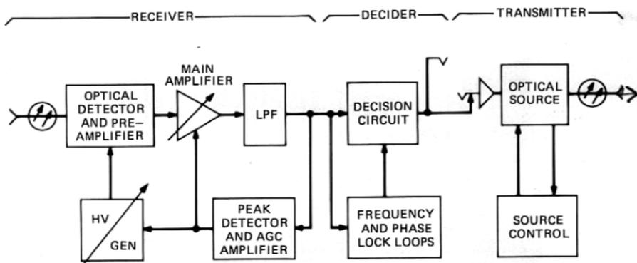
Fig. 2 — Optical regenerator.
