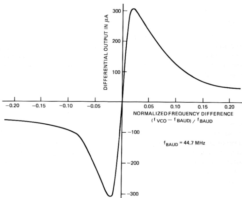
Fig. 16 — Typical frequency comparator characteristic.
