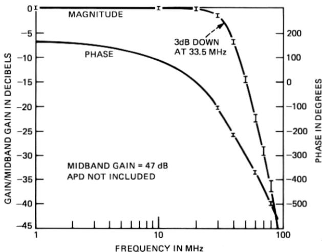
Fig. 7 — Receiver high-frequency electrical gain characteristic.
