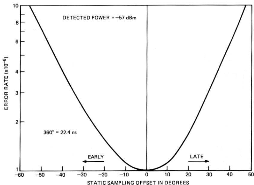
Fig. 13 — Error rate dependence on sampling time.
