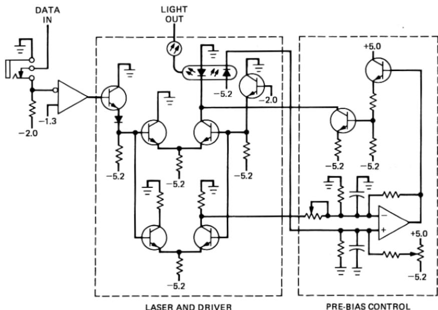
Fig. 18 — Transmitter circuit.
