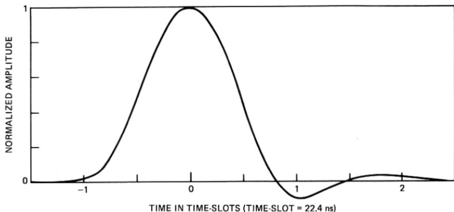
Fig. 9 — Nominal linear channel pulse response.
