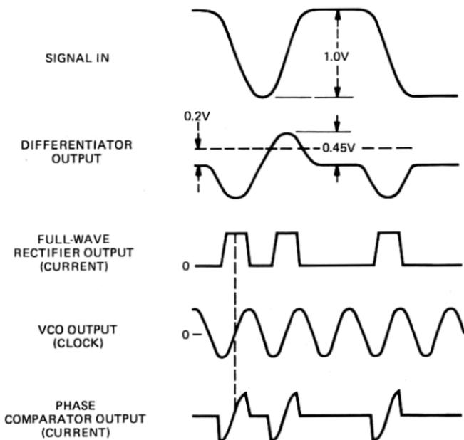
Fig. 15 — Timing recovery waveforms.
