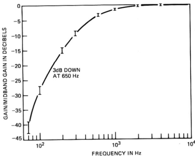
Fig. 8 — Receiver low-frequency electrical gain characteristic.
