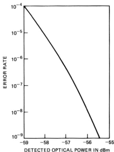
Fig. 5 — Error rate versus detected optical power.
