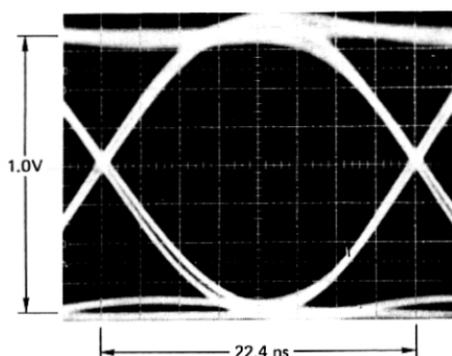
Fig. 10 — Typical eye pattern (receiver output).
