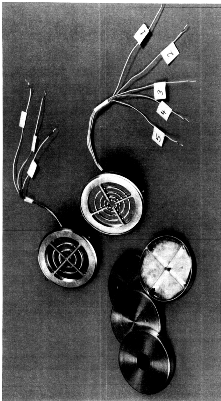
Fig. 6—The experimental 4-bit and 6-bit digital receivers, the acoustic desampling filter, and the earpiece cavity.
