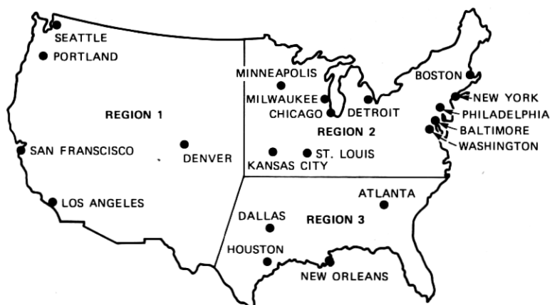
Fig. 3—Three regional maps of the United States. Regional boundaries are selected such that an attenuation curve for a representative ground station in each region applies throughout that region.
