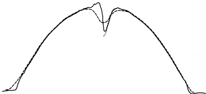
Fig. 18—Profiles of fiber no. 5 as measured by RNF (solid), FOCUS (dotted), and TRANS (broken) techniques.
