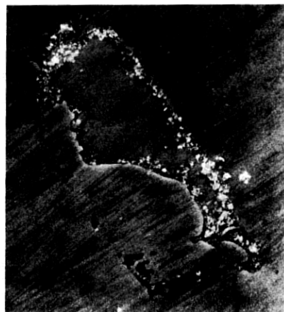
Fig. 11—Indium inclusion on epitaxial layer. (a) Optical. (b) Electron. (c) Acoustic.
