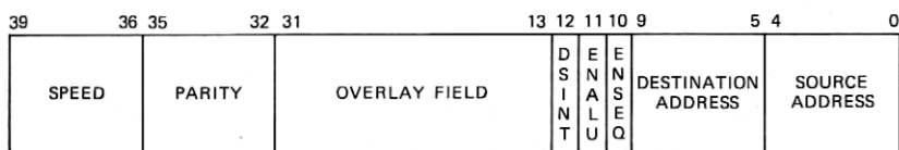
Fig. 8—Microinstruction of the peripheral interface controller.
