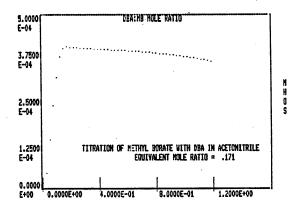
0.0996 N MB. 0.0991 DBA. Pt ELECTRODES, 1 KZ. MED. PAR. AVE. 25.0 C
