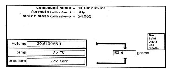
**Figure 4. Converting Units.** Clicking on the 53.4 grams next to sulfur dioxide (Figure 3, "After Rxn" side) brings up a card with pertinent information transferred. Clicking on "Gas" (upper right) brings up the boxes shown. Entering 33 for the temperature and 772 for the pressure and then clicking the bottom arrow with the "Sig Figs" button unhilited leads to the result shown (20.6..... L).
