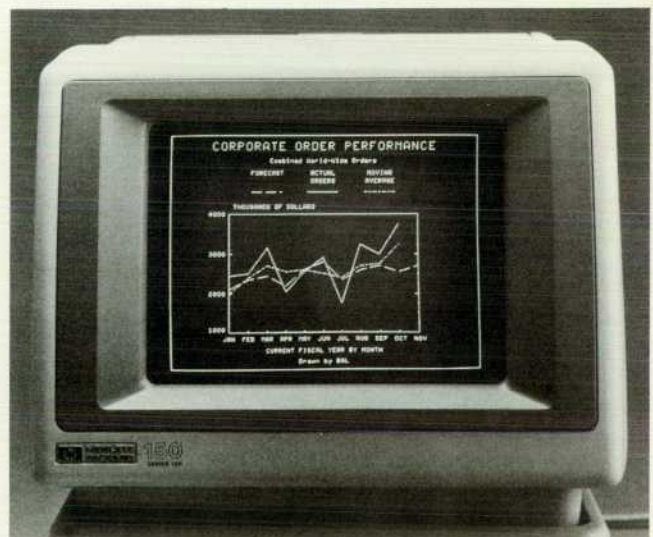
Fig. 4. The graphics display has a resolution of 512×390 pixels.
